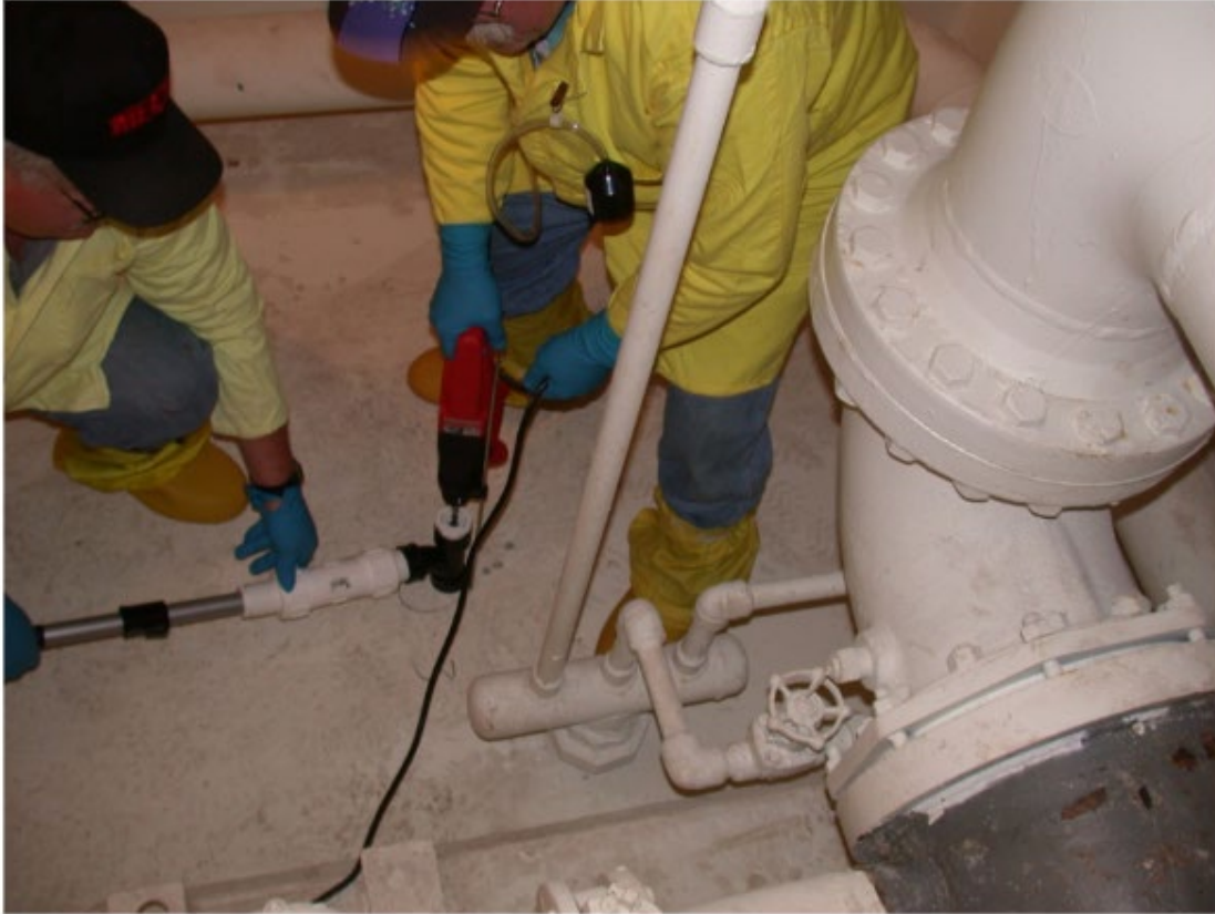
Image: concrete dust sampling, EPRI 3002005412
