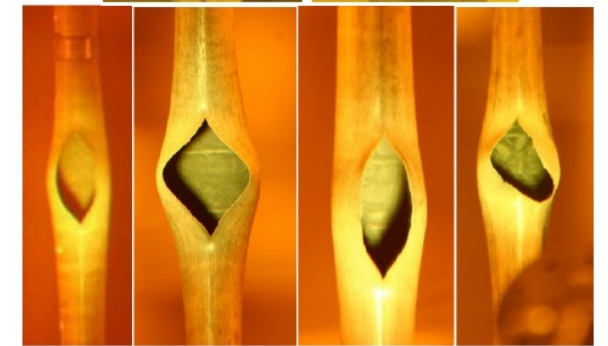
Burst openings from Studsvik LOCA tests (NUREG-2121)
