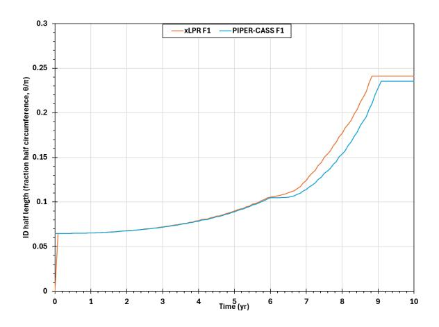
Benchmark inputs chosen to yield artificially fast fatigue crack growth
