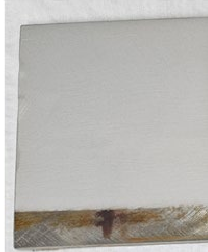
Ceramic Zirshot performed best in initial testing (4 RPM, 50 um, 0°)
