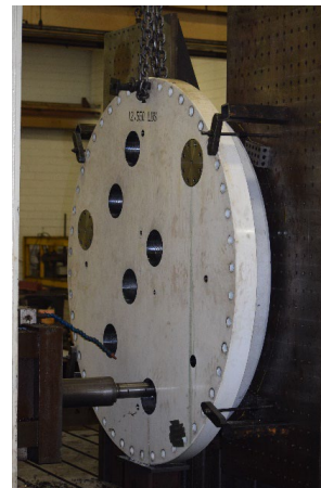
Machining holes in lid
