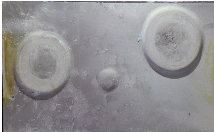
Blistering is only applicable to absorber materials with cladding (i.e., Boral, Maxus, etc.)
