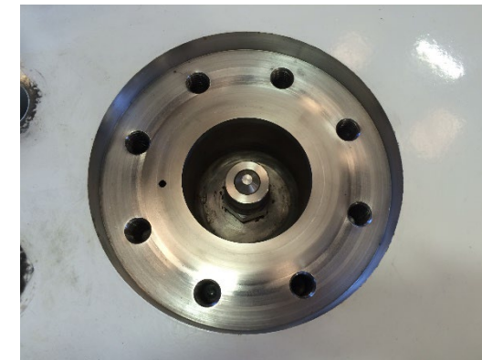
Vent port with quick-connect
