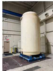
TN-32B cask at EPRI
