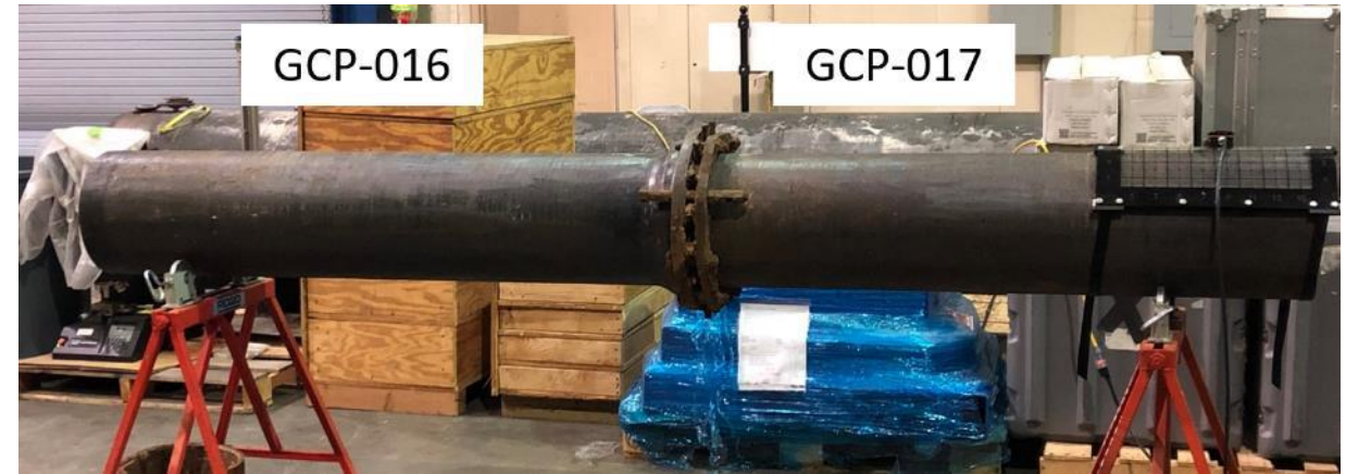
EPRI Samples GCP-016 & GCP-017 after wire-brush cleaning (no visually detectable wall loss)
