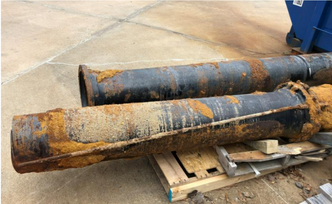
EPRI Gray Cast Iron Pipe Sample GCP-016 on-arrival Diameter: 12-inch (30 cm) Length: ~65-inch (1.7 m)
