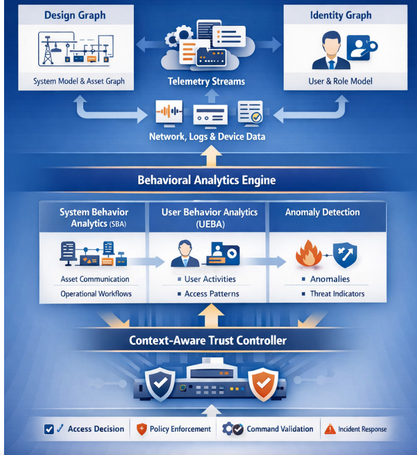
Figure 1: EPRI's ZT4OT Security Architecture showing Design Graph, Identity Graph, Telemetry Streams, Behavioral Analytics Engine, and Context-Aware Trust Controller.
