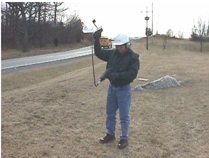
Figure 2-3 Technician Using Ultrasonic Concentrator to Detect Ultrasonic Emissions from Overhead System
