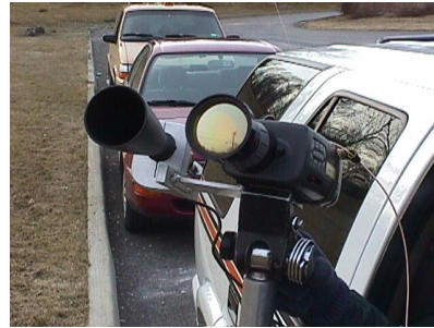
Figure 2-2 Ultrasonic Long Range Module (Horn) on Left Infrared Camera on right
