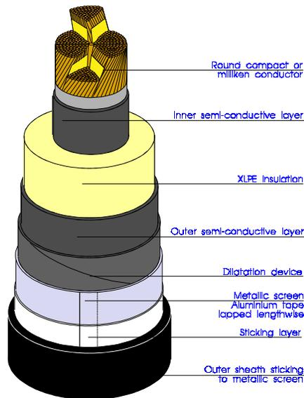
Figure 4 : New technical step of 90 kV cable
