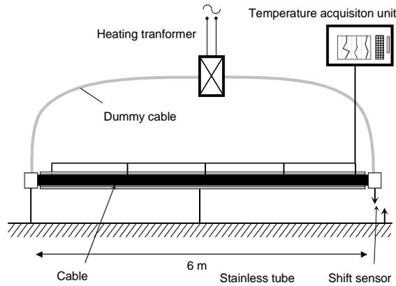
Figure 1 : Elongation test bench
