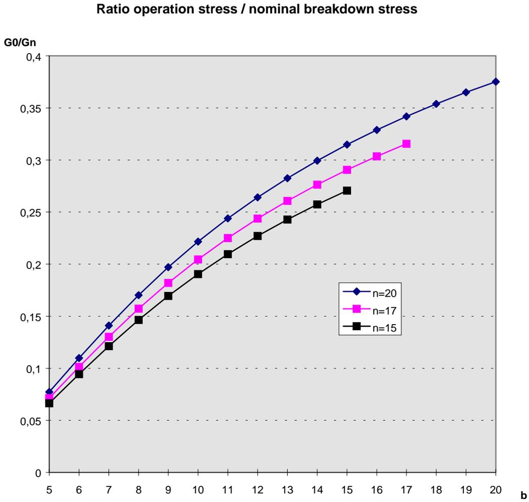
Figure 1 : ratio of the allowable operation stress upon the nominal breakdown stress
