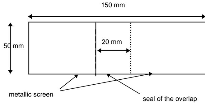
Figure 11 : overlap seal test
