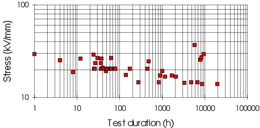
Figure 6 : joints a.c . withstand test results
