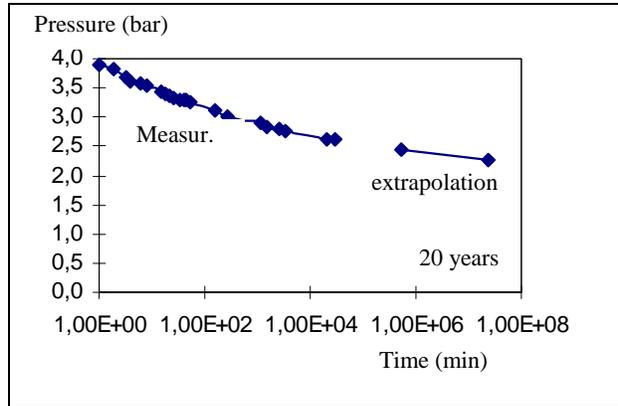
Figure 5 : Measurement and extrapolation, by means of Thirion and Chasset model, of the hoop pressure of the insulating interface on a period of 40 years, m = 0.1.
