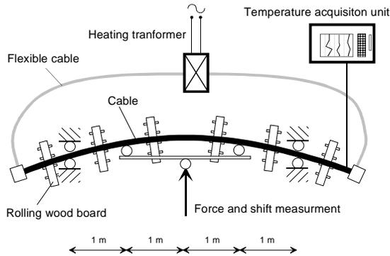
Figure 5 : Flexural rigidity test bench
