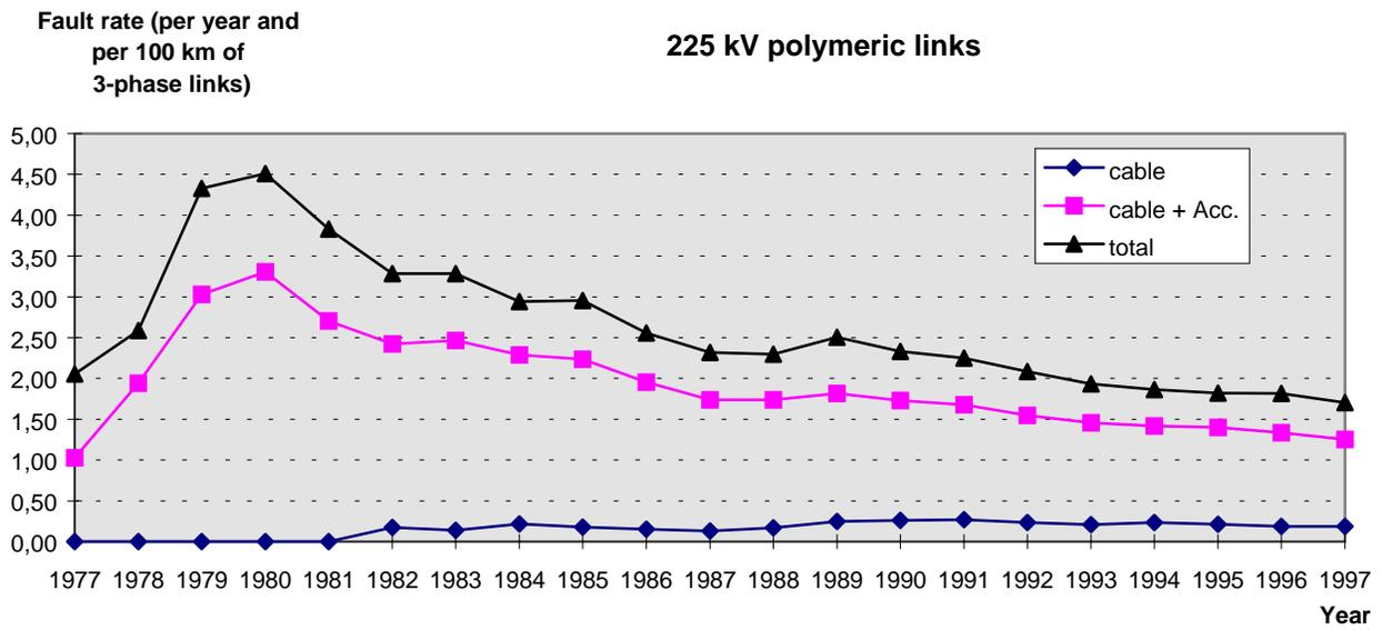
Figure 3 : Fault rate of polymeric underground links
