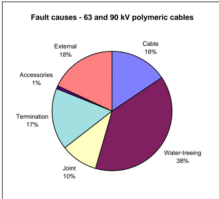
Figure 2 : Fault causes
