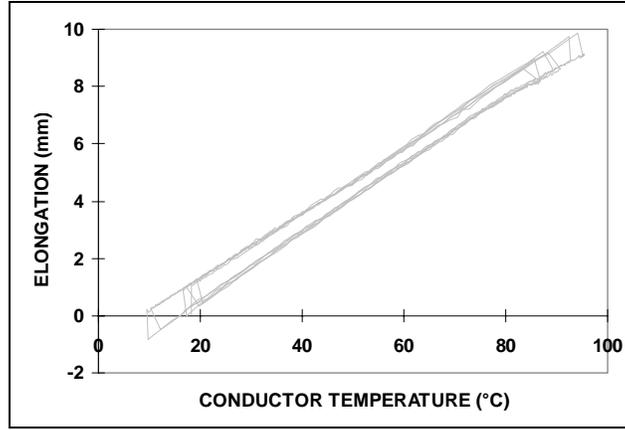
Figure 2 : Results of the cable elongation during heating cycles
