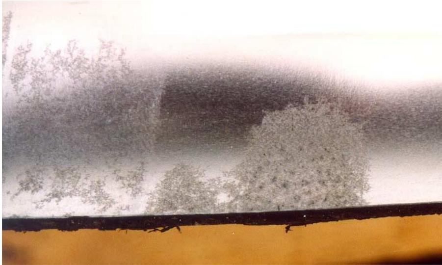
Figure 14 : Screen Corrosion
