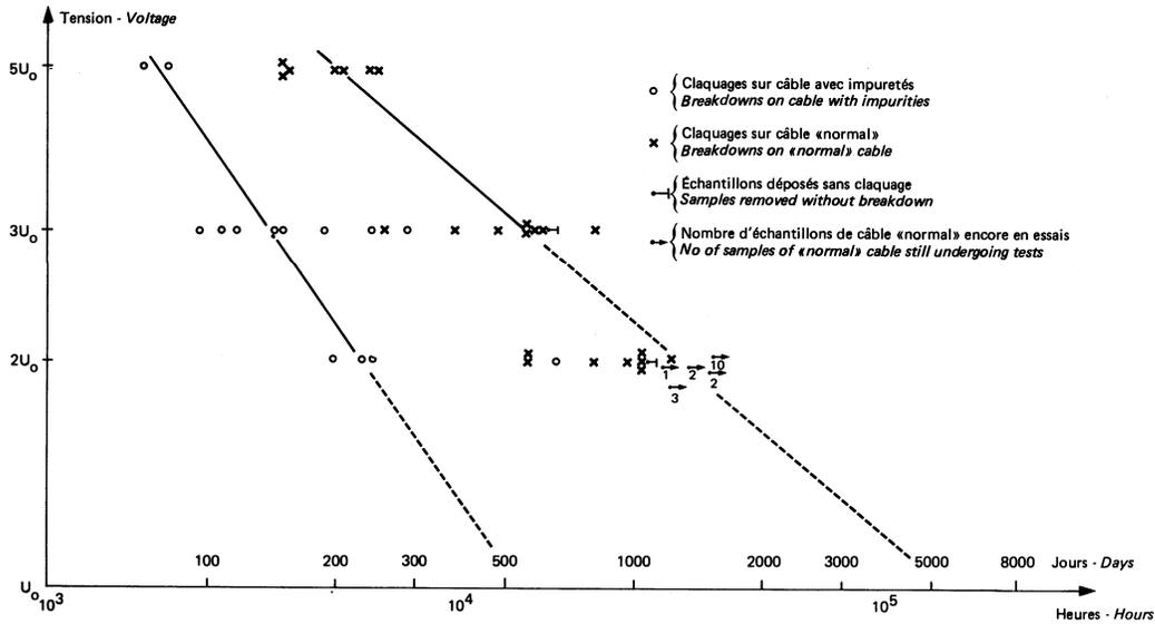
Figure 2 : Lifetime of cables with water in the conductor.
