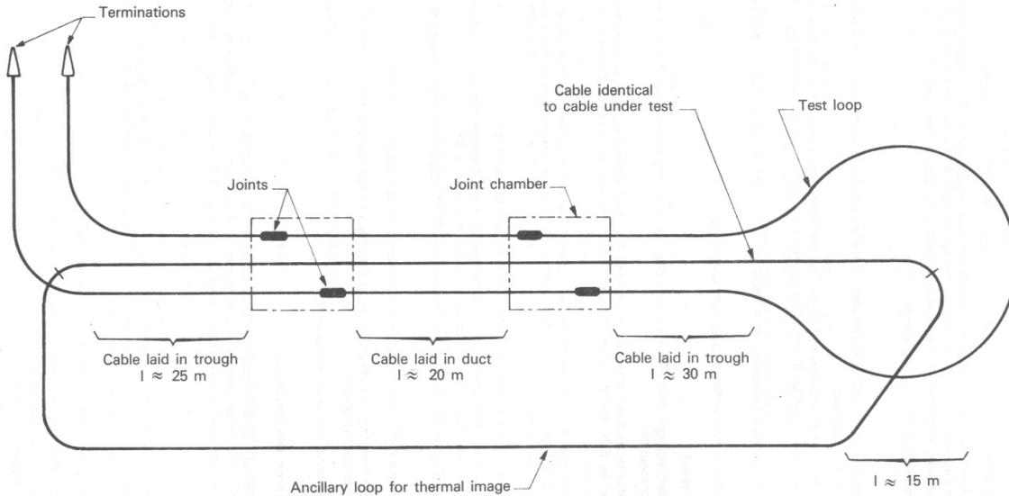
Figure 7 : Installation for long duration test
