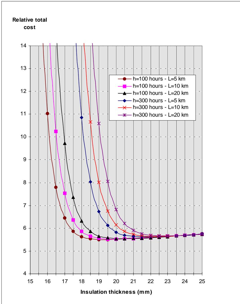
Figure 7 : Total cost of underground 225 kV transmission as a function of insulation thickness of cables.
