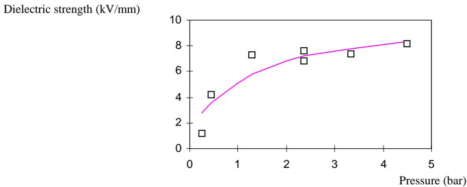
Figure 4 : Test on the dielectric strength of the interface (for given preparation and materials).
