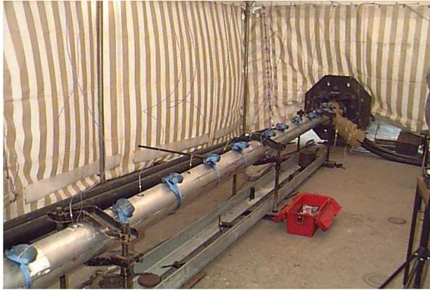
Figure 3 : Mechanical test bench for axial force measurement
