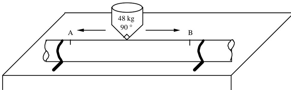
Figure 8 : Abrasion test - principle
