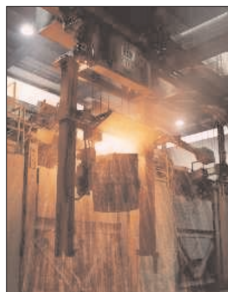
Figure 1. Tapping a 30,000 kg capacity channel induction furnace
