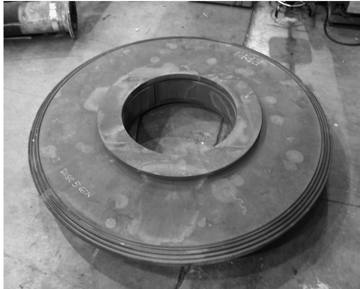
Figure 8 - Retired Disk with Cracking
