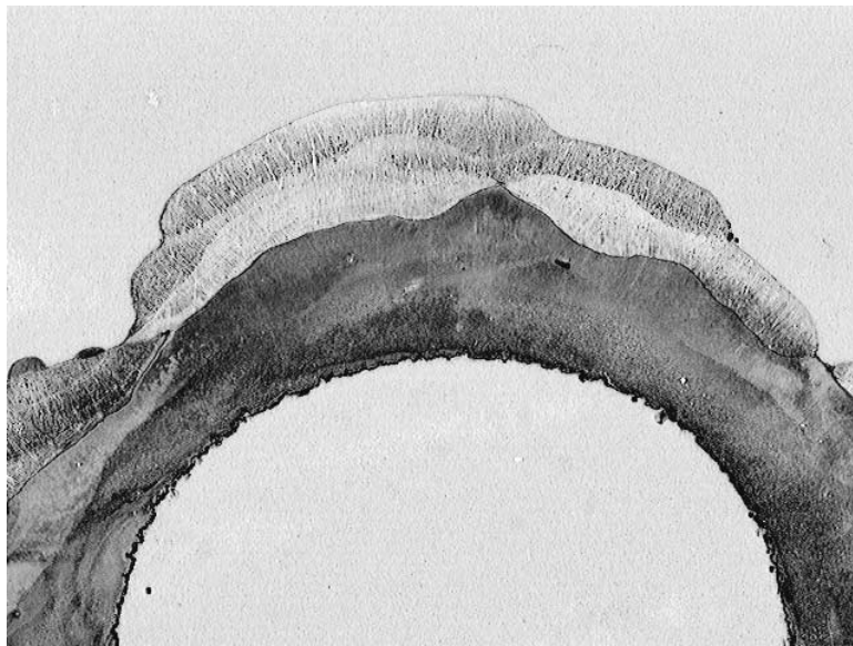
Figure 5-3 Cross section of overlaid tubing with incomplete coverage
