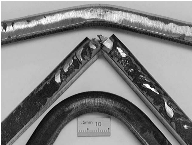
Figure 7-1 Weld overlay tests after tempering and bending
