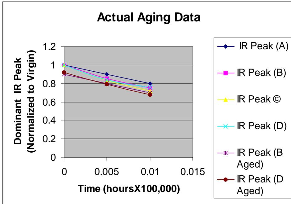
Figure 6-1 shows that the actual aging data from the 500 hour low conductivity test and 1000 hour (30,000 cycle) rotating wheel test.
