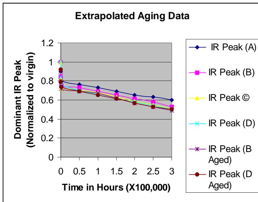
Figure 6-2 shows the extrapolated graph based on the actual data. Acknowledging the risks of extrapolation based on limited testing, the figure nevertheless indicates that the insulators can be expected to perform satisfactorily over a 30 year (262,000 hours) life.
