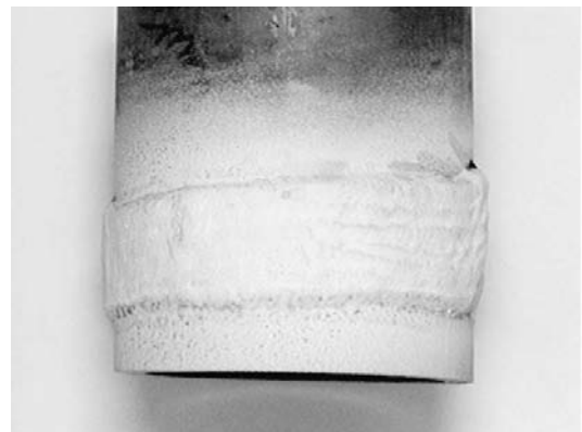
Figure 3-4. Liquid Penetrant Test – NOREM-02A/Type 304 SS 4-in. schedule 80
