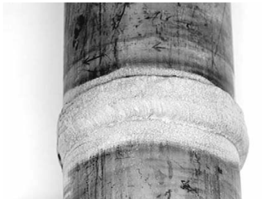
Figure 3-3. Liquid Penetrant Test - Stellite 21/Type 304 SS 4-in. schedule 80 (narrow oscillation, <0.25-in.)
