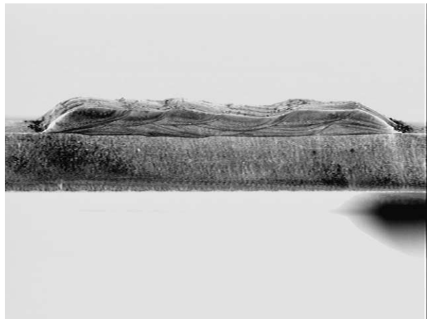
Figure 3-10. 5x examination at 180 degrees location (top) – Norem-02A
