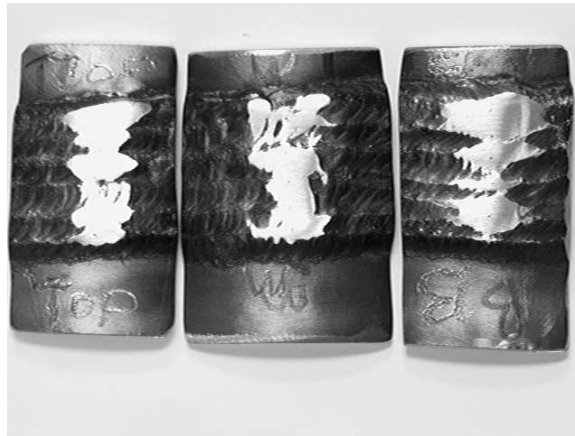
Figure 3-5. Typical surface preparation and location for Hardness measurements per QW-462.5 (b).
