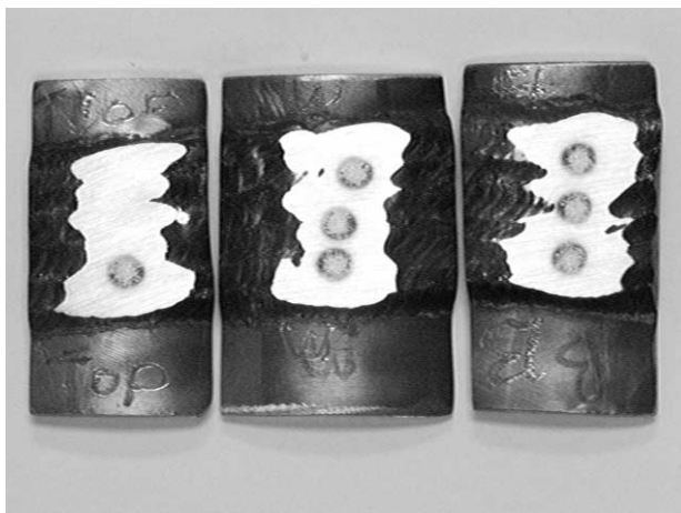
Figure 3-13. Typical surface preparation and location of chemistry analyses.
