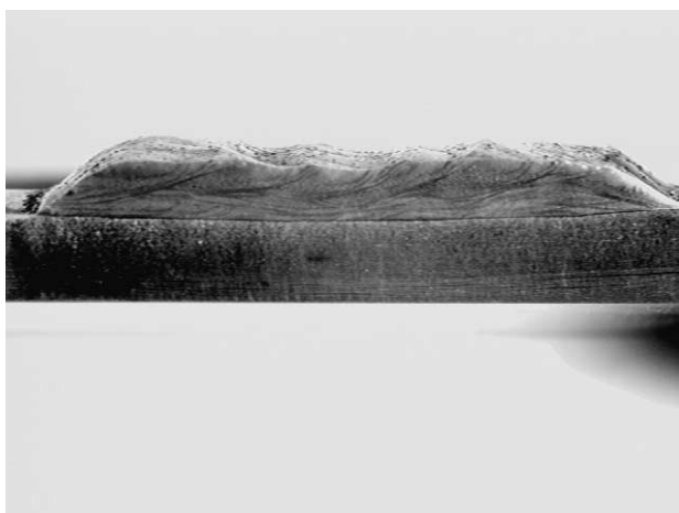
Figure 3-12. 5x examination at 0 degrees location (bottom) – Norem-02A
