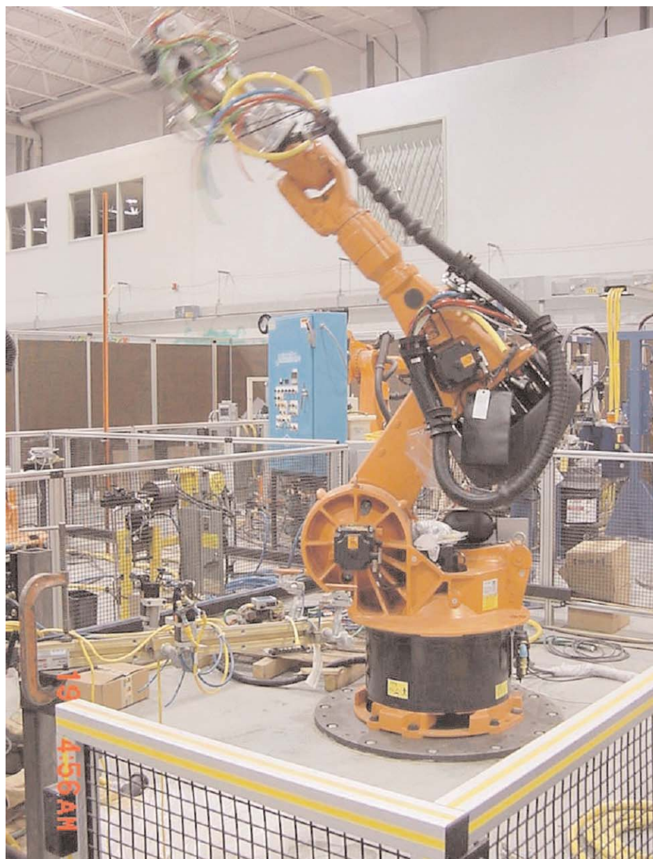
Figure 1. Robot In Motion During Voltage Sag Testing (Courtesy Kuka)
