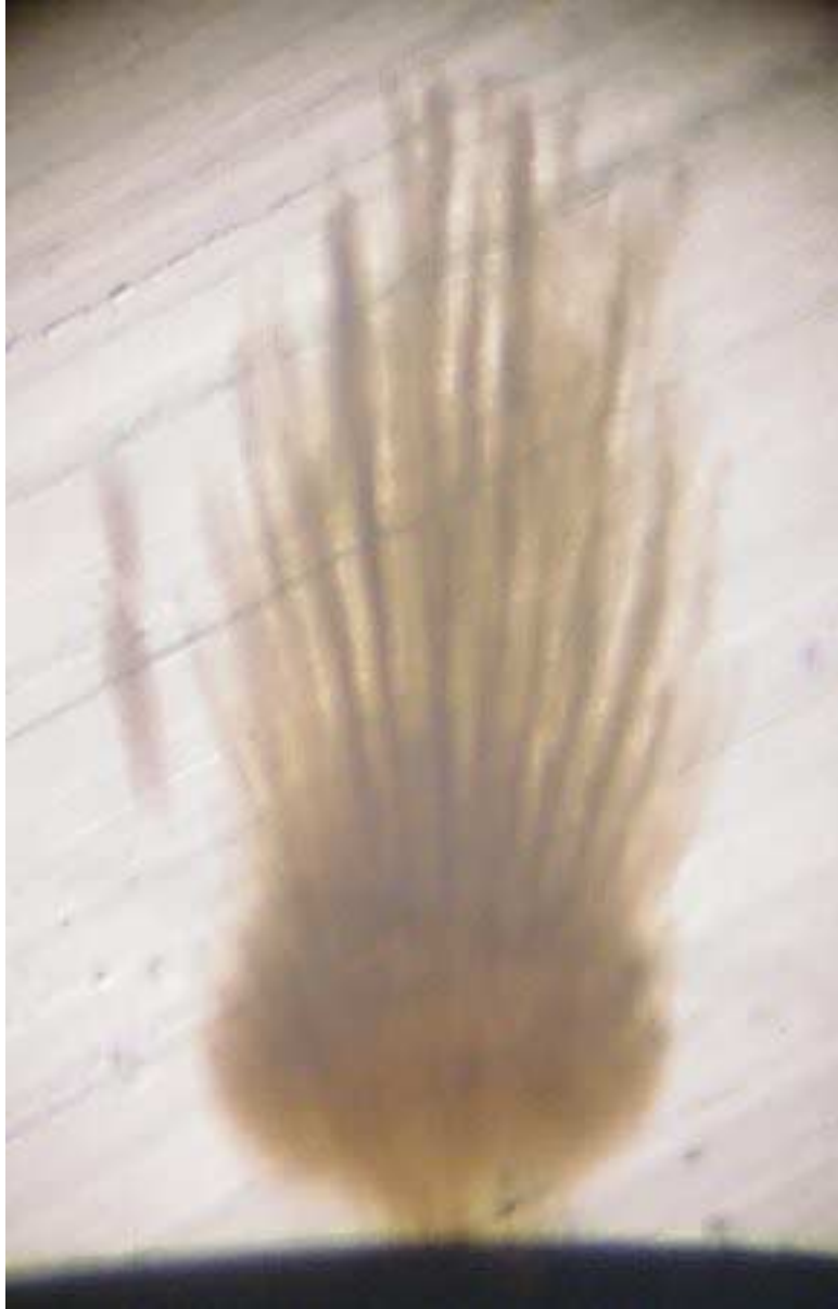
Figure A-1 Typical vented water tree growing from conductor shield. Note bow-tie tree on left hand side
