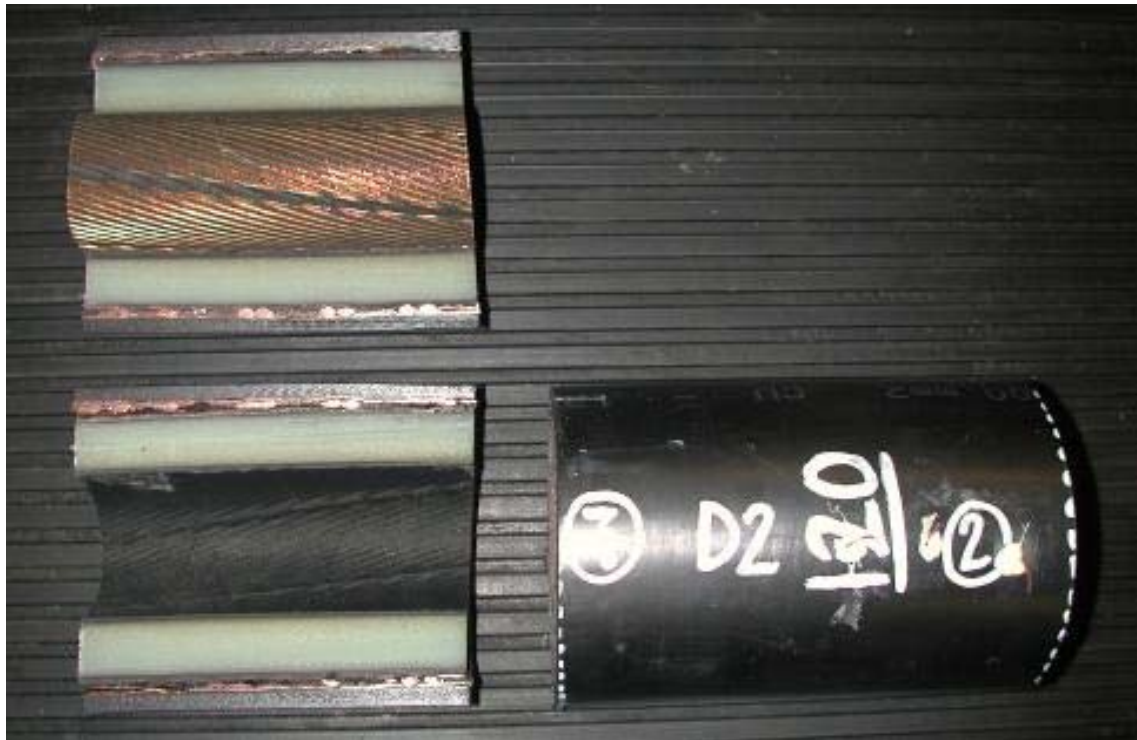
Figure 6-15 Dissected Copper Foil Laminated Cable with Jacket and Neutral Wires in Place
