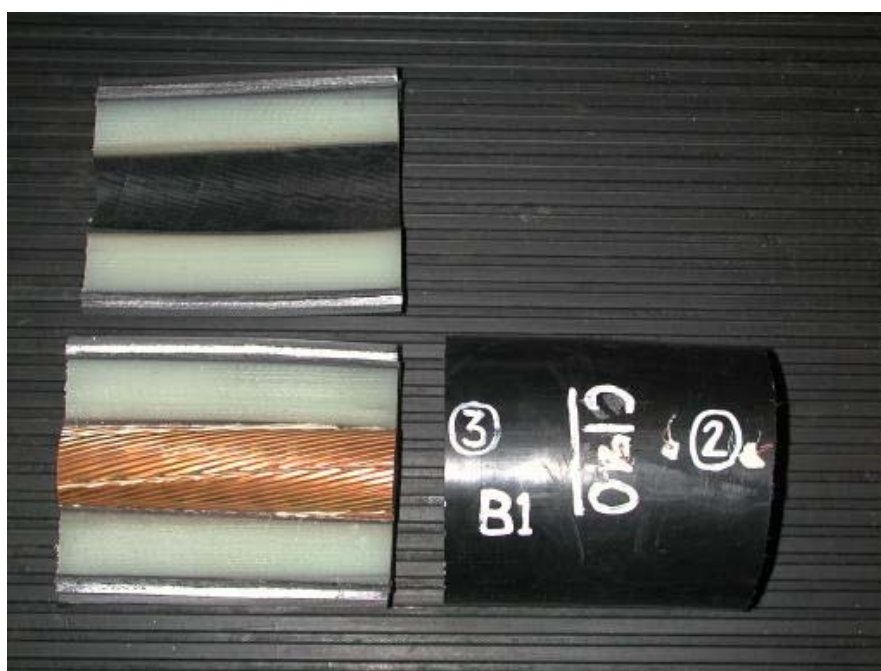
Figure 6-10 Dissected Lead Sheathed Cable Sample After the Clamping Test
