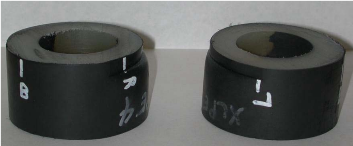
Figure 4-3 Photos of Samples After Testing, Showing Permanent Deformation (313 kPa Sample on the Left, 162 kPa Sample on the Right)
