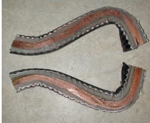
Figure 6-7 A Photograph of the Dissected Cable at the Sharp Bend
