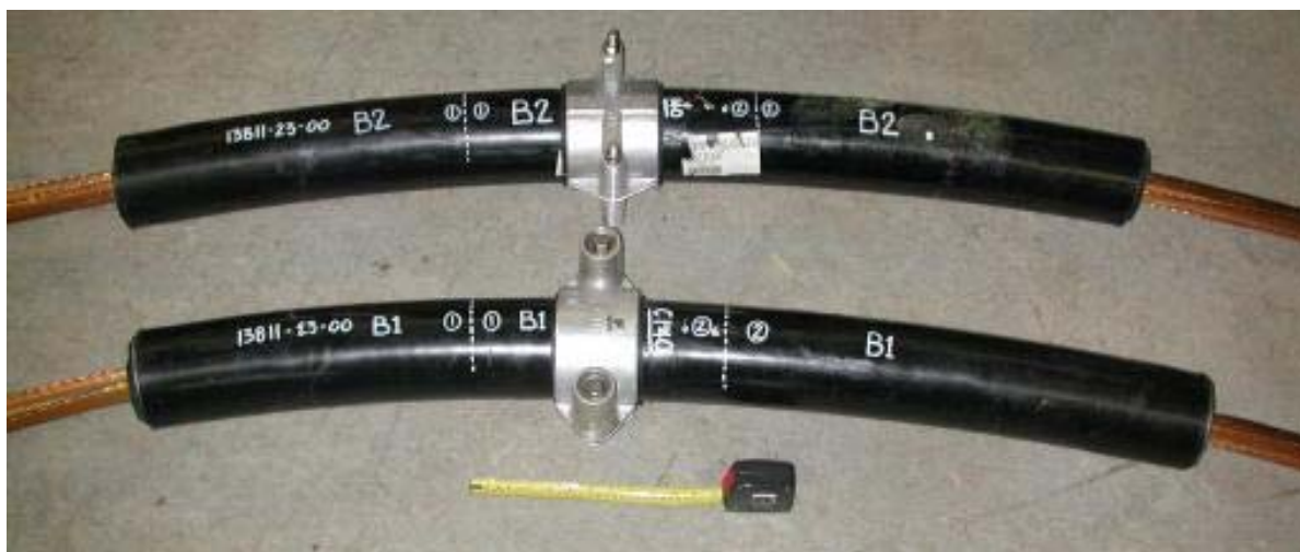
Figure 6-9 Lead Sheathed Cable Samples After the Test, Ready for Dissection
