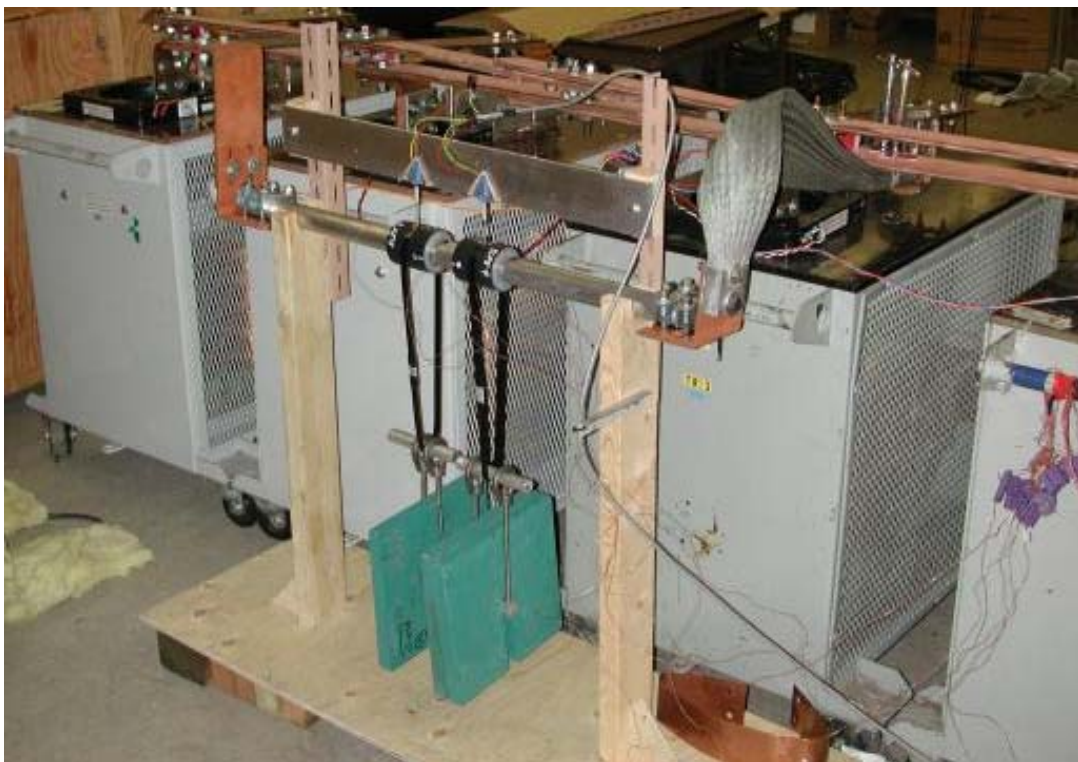
Figure 4-4 The Test Setup for Loaded Temperature Cycling
