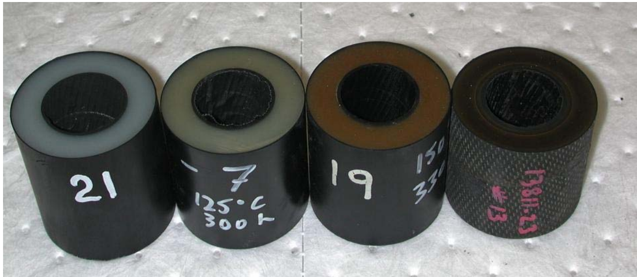
Figure 5-3 Progressive Darkening of Thermally Aged XLPE Samples (Left to Right): Not Aged, Oven Aged 300 Hours at 125°C, Oven Aged 330 Hours at 150°C, and Cycled for 2450 Hours at up to 150°C
