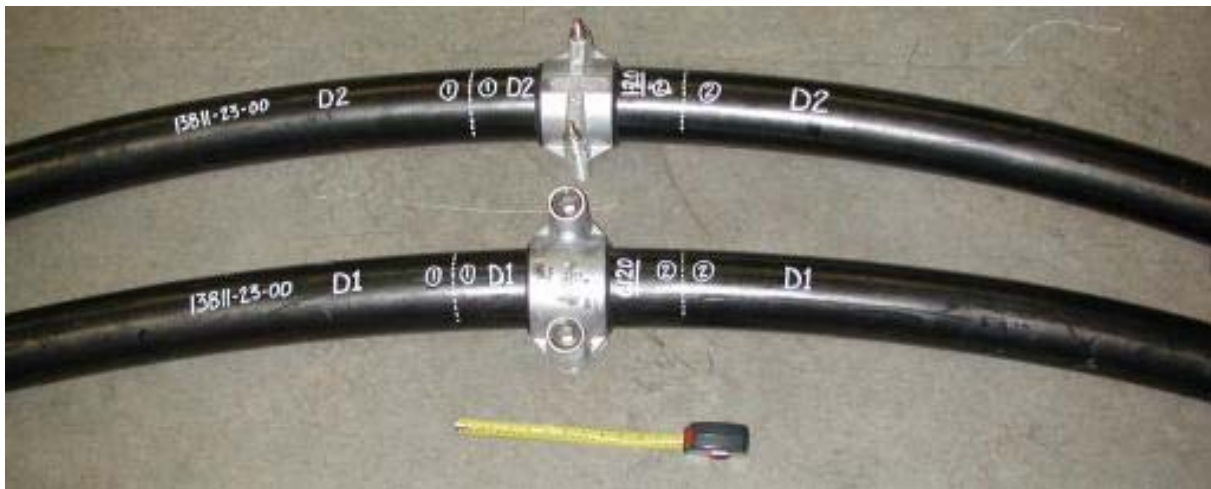
Figure 6-13 Copper Foil Sheathed Cables After the Test, Ready for Dissection
