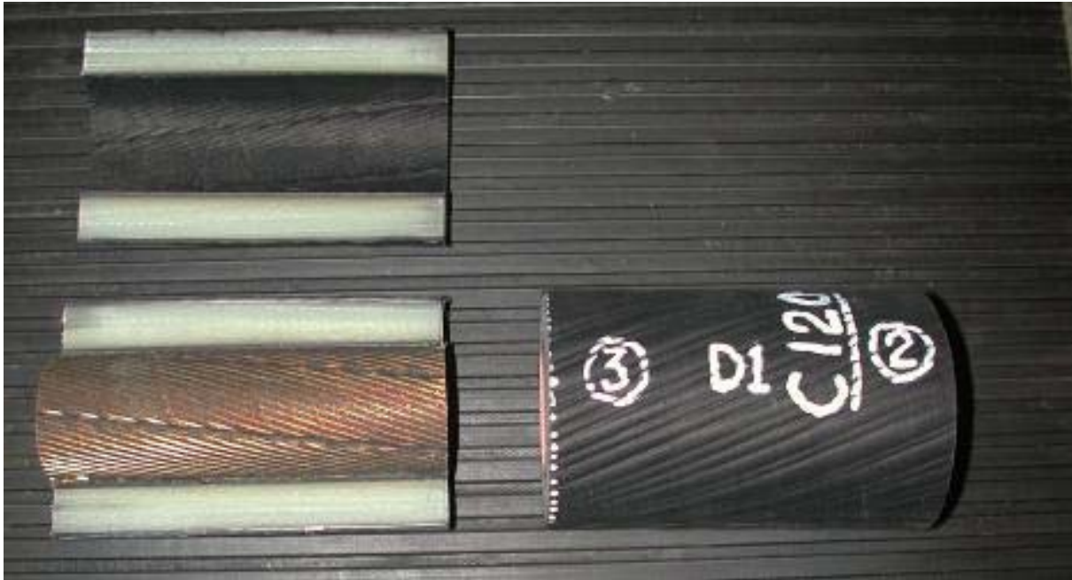
Figure 6-14 Dissected Copper Foil Laminated Cable with Jacket and Neutral Wires Removed
