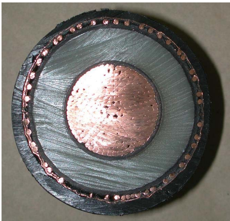
Figure 6-16 Cross Section Photo of Cable D2 Under the Center of the Clamp After the Test
