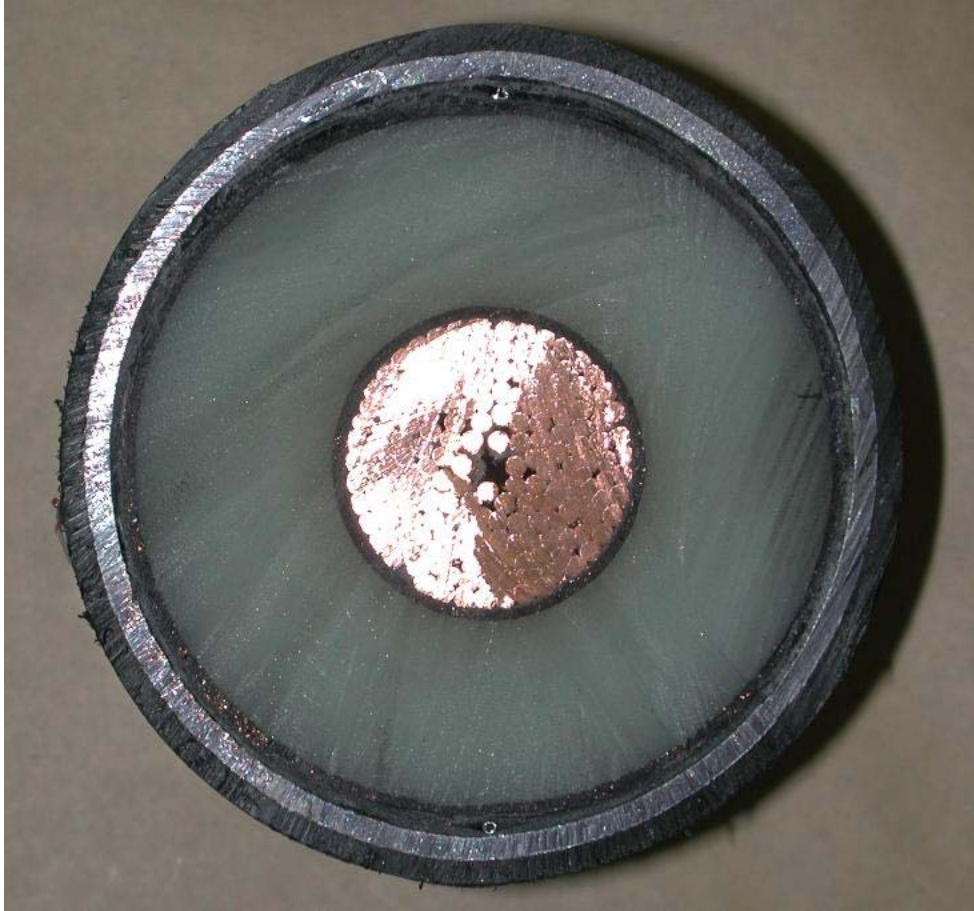
Figure 6-11 Cross-Section Photo of Cable B1 Under the Center of the Clamp After the Test
