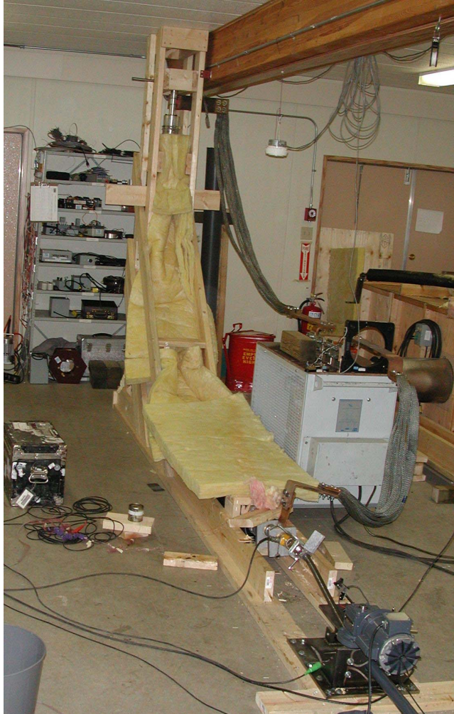
Figure 6-2 Photograph of the Minimum Bending Radius Test Setup
