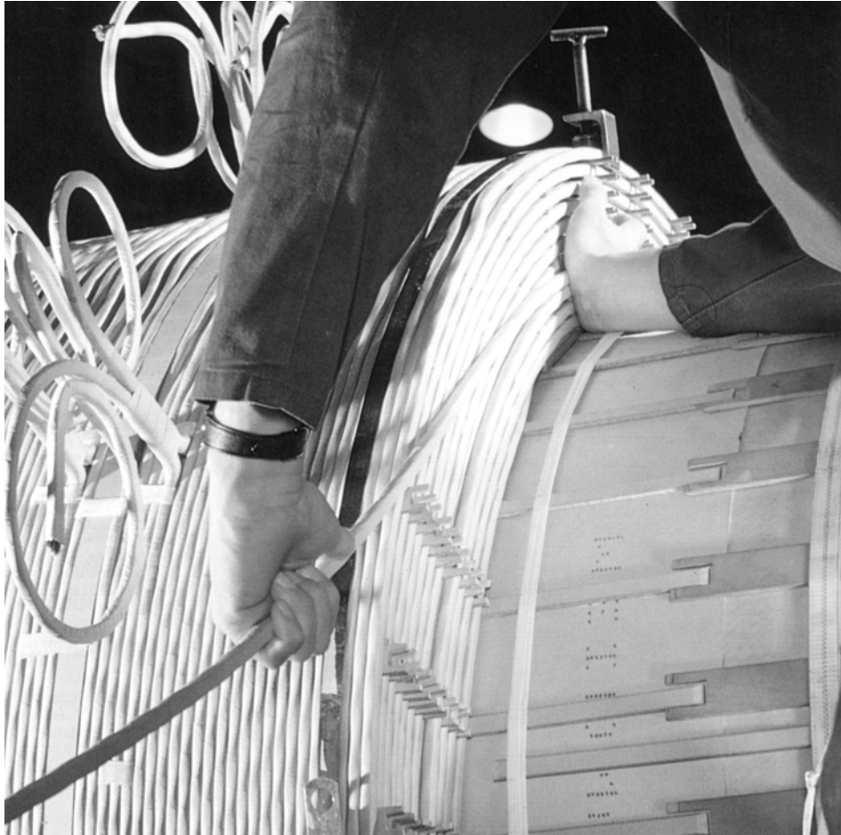
Figure 3-10 Construction of Cylindrical Windings (Courtesy of SMIT)
