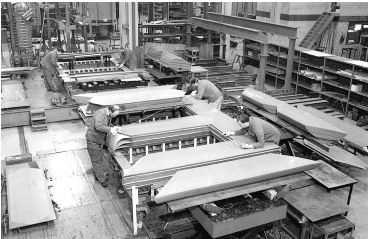
Figure 3-5 Construction of Laser Cut Core Laminations (Courtesy of SMIT)
