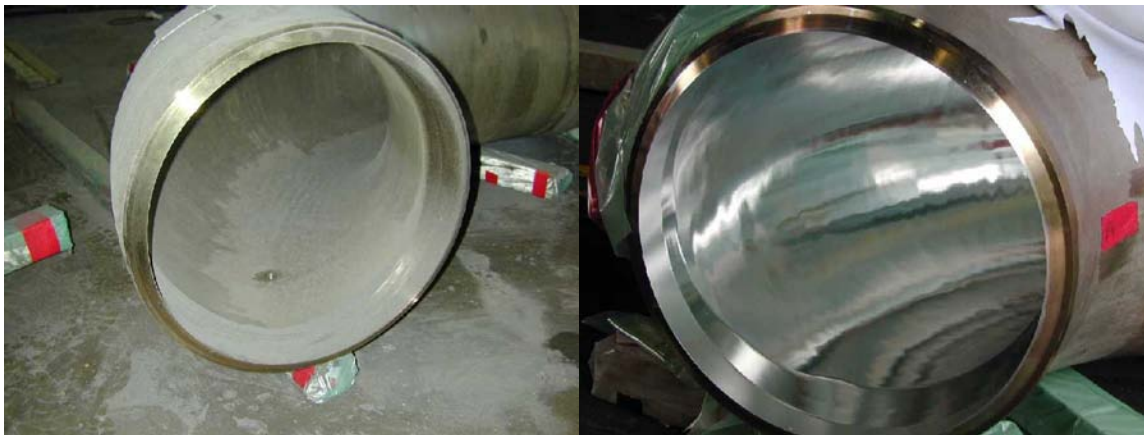
Figure 4-1 Comparison of “As-Received” and Electropolished Surfaces (28\" elbow)
