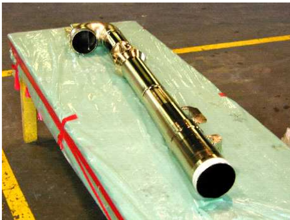
Figure 4-14 Jet Pump Following Application of SCrP
