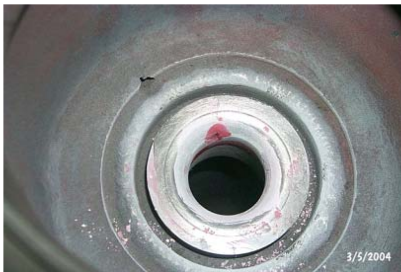
Figure 3-1 Stellite Valve Seat Damage
