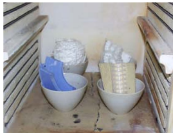
Step 2: Ash in Lab Oven
