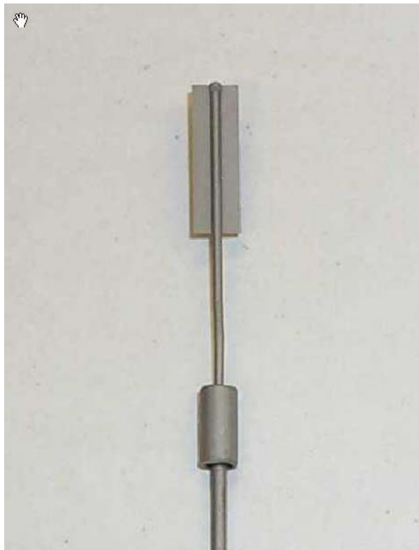
Figure 2-1 Schematic of Weldable Resistance Gage (Source: Tokyo Sokki Kenkyujo Co.)
