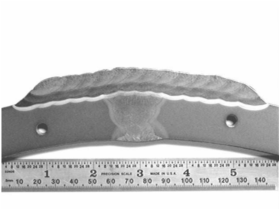
Figure 2-2. Cross section of Weld Overlay
