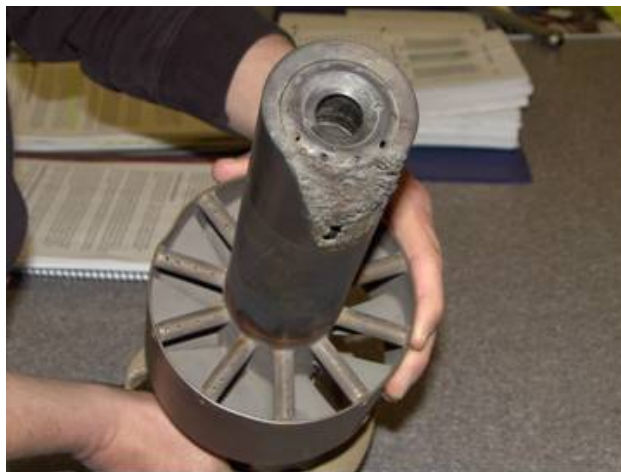
Figure 6-1 Nozzle Tip Burnout due to Flashback
