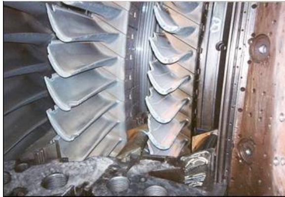
Figure 6-4 First and Second Stage Blade Damage from CD-Induced Failure of S/W 501F Transition Pieces
