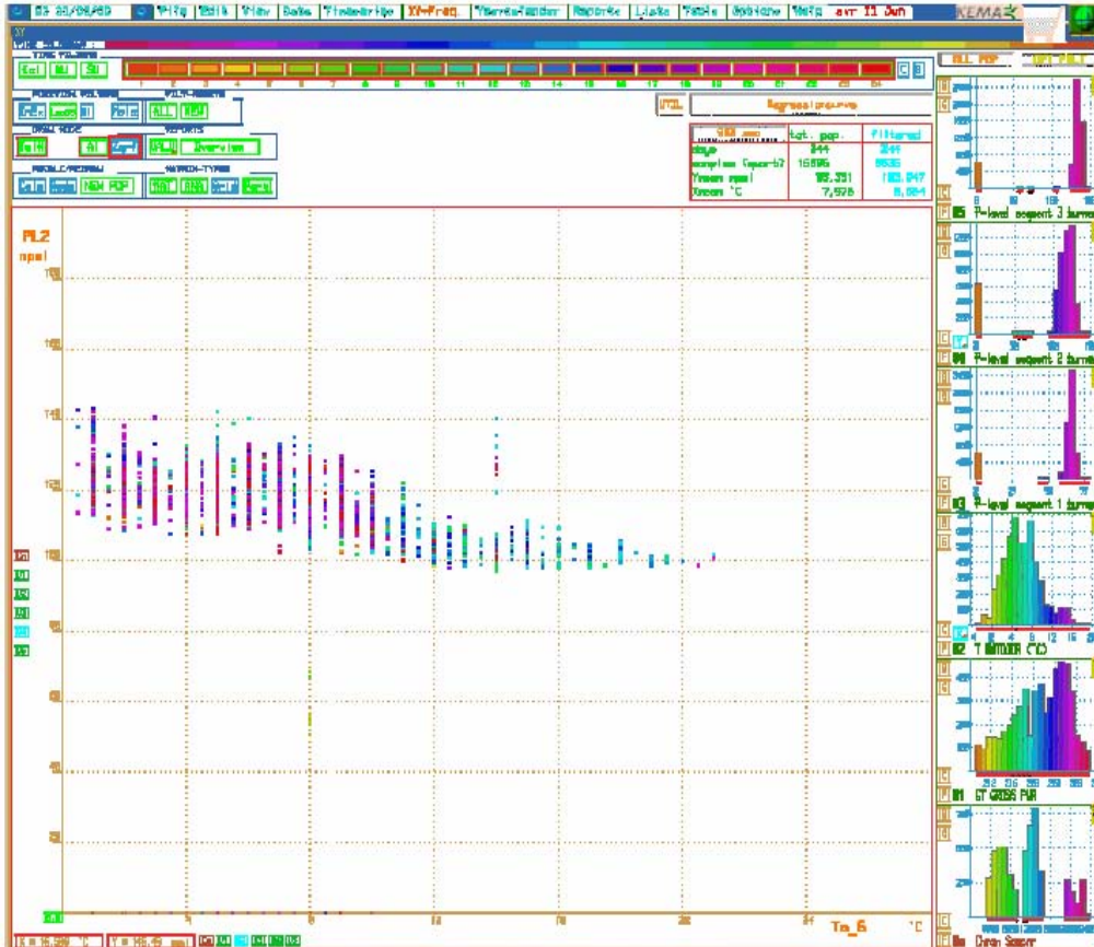
Figure 2-18 Analysis of CD Pressure Amplitudes with Changes in Ambient Temperature at Constant Engine Load
