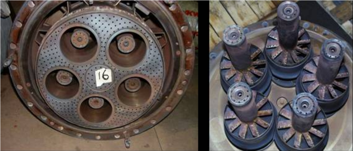
Figure 3-8 Upstream Part of the Combustion Chamber with the Outlet of the Five Premix Burners and Embedded Diffusion Burners. The Burners are also Shown Separately.
