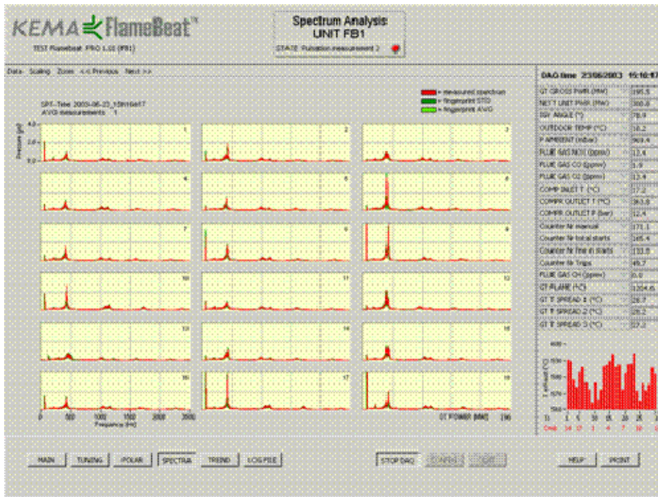
Figure 2-12 FFT Dynamic Spectra of 18 Combustion Chambers of the GE MS 901FA Gas Turbine, Recorded with FlameBeat™
