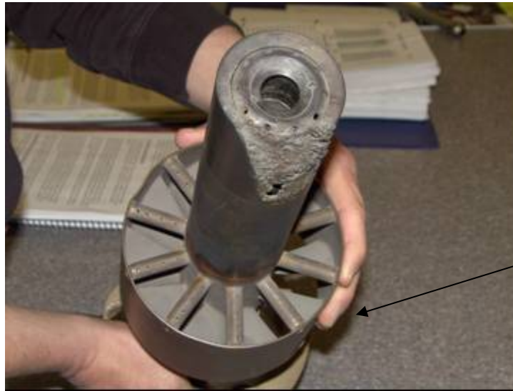
Figure 1-3 Nozzle Tip Burnout due to Flashback
