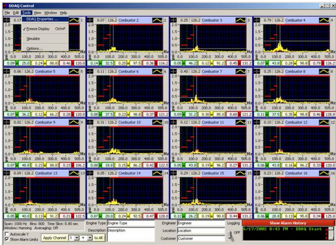
Figure 2-16 Display Screen for Individual Combustor Dynamic Spectra in Relation to Alarm Set Points – PSM DAAQ Display
