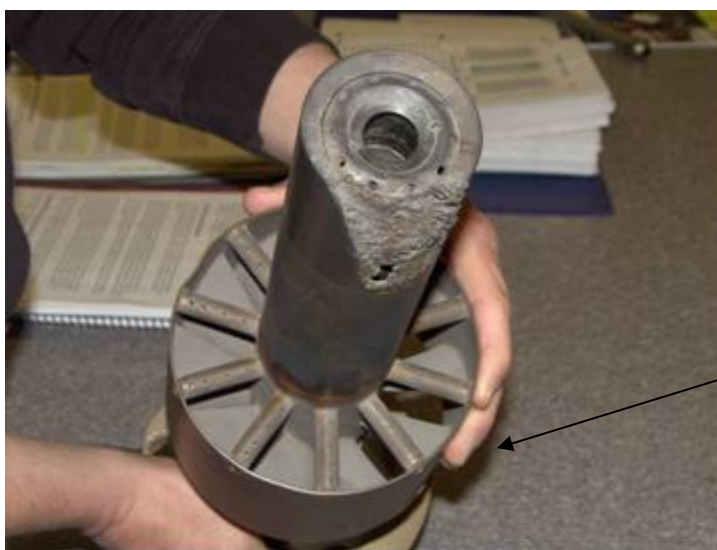
Figure 1-3 Nozzle Tip Burnout due to Flashback
