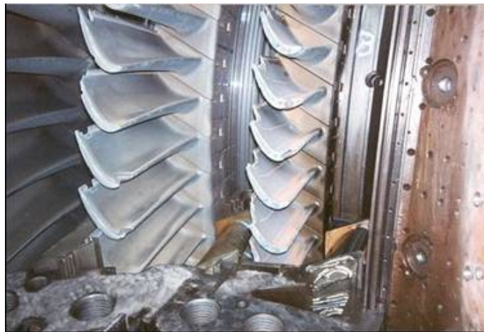
Figure 1-6 First and Second Stage Blade Damage from CD-Induced Failure of S/W 501F Transition Pieces
