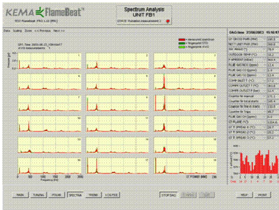
Figure 2-12 FFT Dynamic Spectra of 18 Combustion Chambers of the GE MS 9001FA Gas Turbine, Recorded with FlameBeat™
