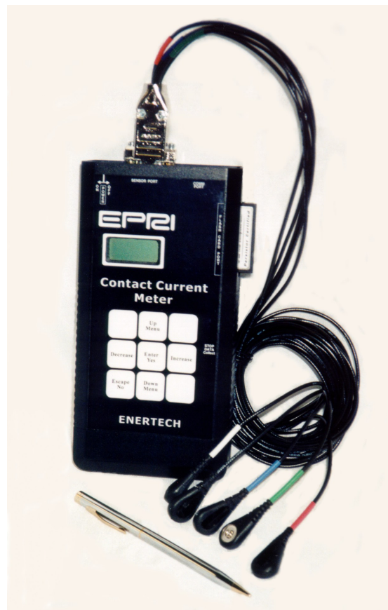
Figure 1-1 The EPRI Contact Current Meter with sensor cable assembly (adhesive sensor connectors not shown)
