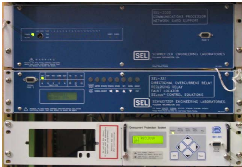
Figure 5-1 SEL 351 and Basler 951 Relays Installed in the Test Stand
