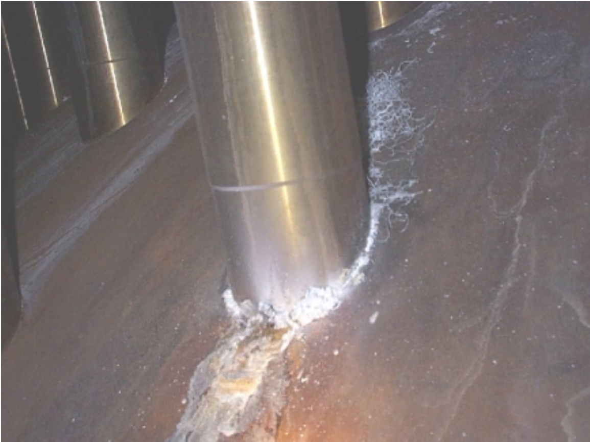
Figure 1-3 Leaking CRDM Nozzle at Oconee 3
