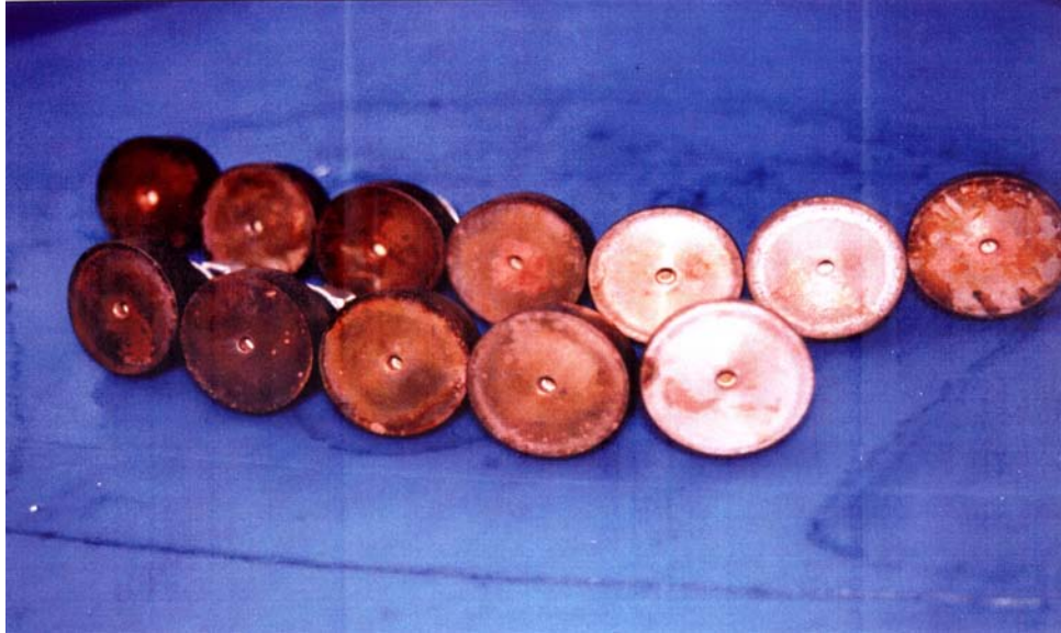
Figure 5-11 New Diverter Switch Contacts for Kent
