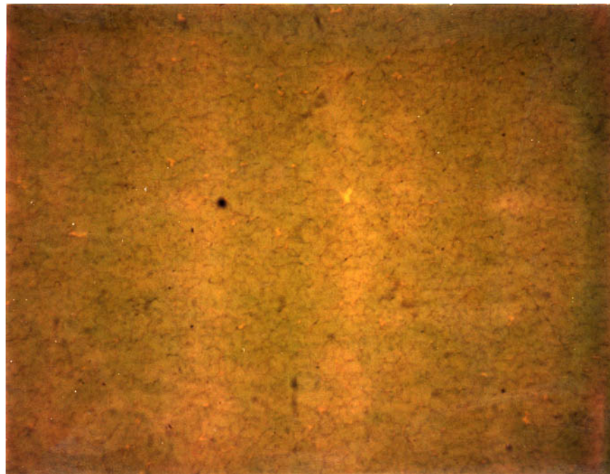
Figure 5-17 Microstructure of Sample #4 in the As-Polished (not etched) Condition (Magnification: 500X)
