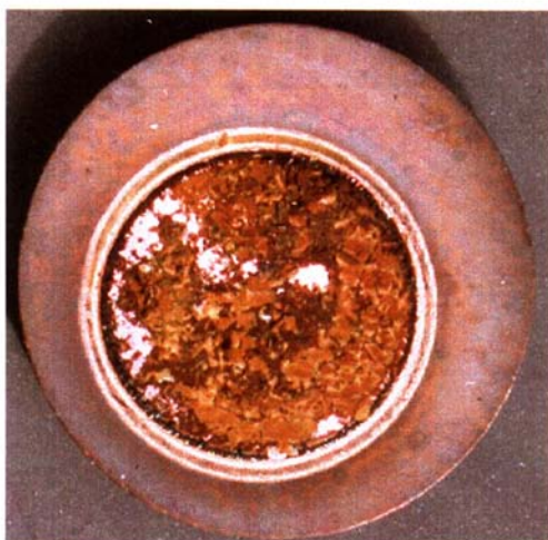
225°C: Old Voltesso-35 (The deposit is flaking off)
