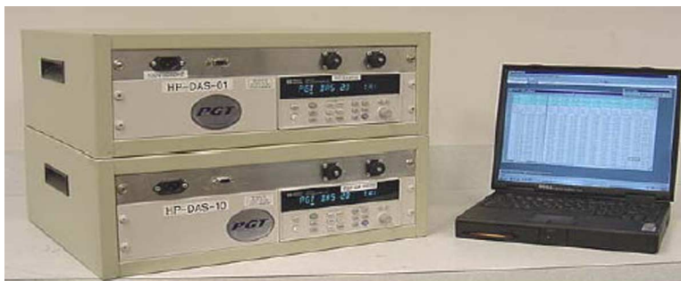
Figure B-8 Power Generation Technologies Data Acquisition System Hardware
