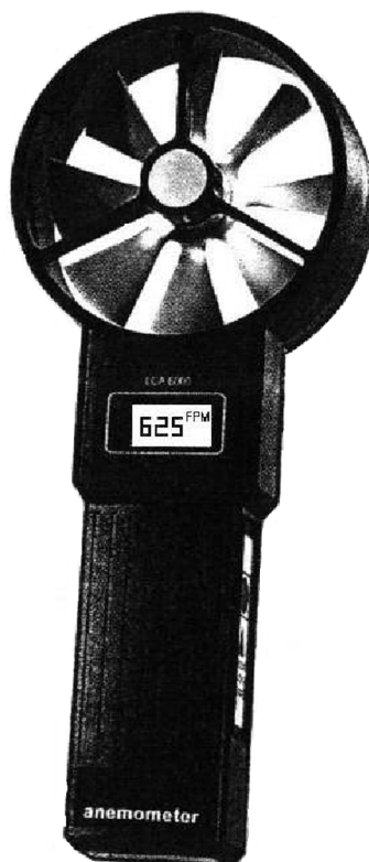
Figure B-2 Typical Electronic Rotating Vane Anemometer
