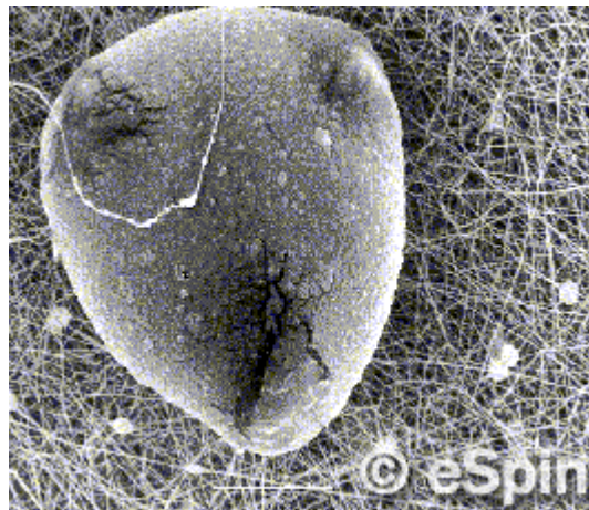
Figure 4-4 eSpin Technologies' Nanofibers (in background) Compared to a Pollen Particle (in foreground)
