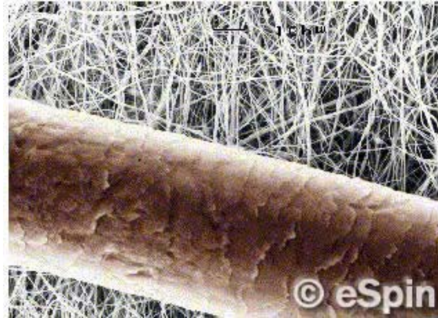
Figure 4-3 eSpin Technologies' Nanofibers (in background) Compared to a Single Human Hair (in foreground)
