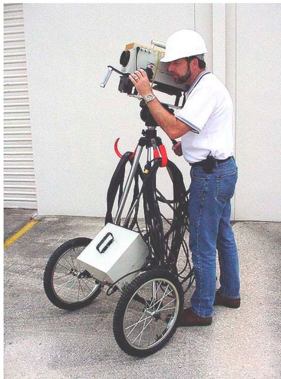
Figure 1. The latest version of the LIS/EPRI SF 6 Camera (TG-30).
