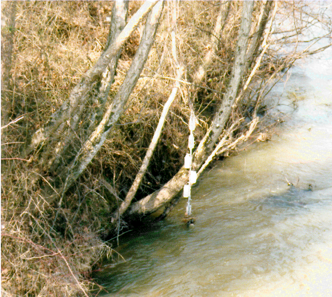
Figure 3-2 Multiple Single Stage Samplers Mounted on a Post for Sediment Sampling
