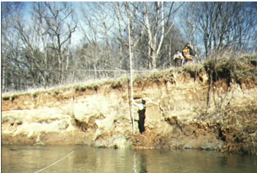
Figure 4-4 A Picture of Measuring Mass Loss of River Bank Erosion in Muddy Creek, North Carolina
