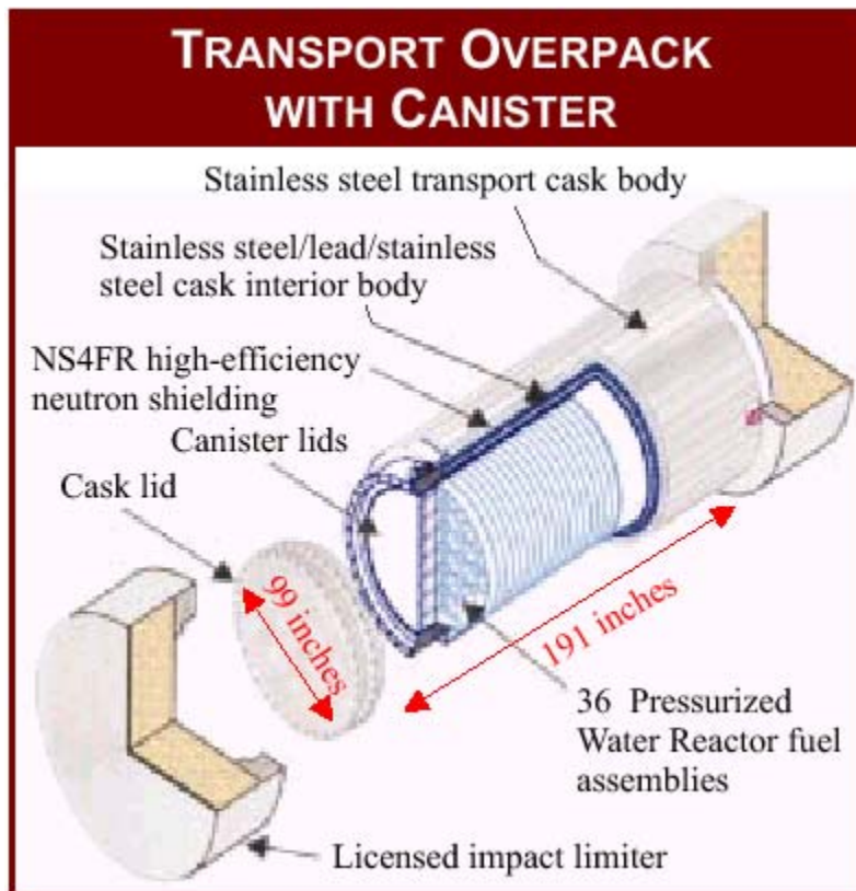
Figure C-1 Transportable NAC-MPC Storage Canister Showing the Spent Fuel Basket
