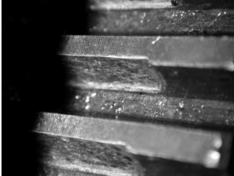
Figure 4-1 Sleeve Wear in a Gear Coupling Courtesy Rota-Tech Inc.
