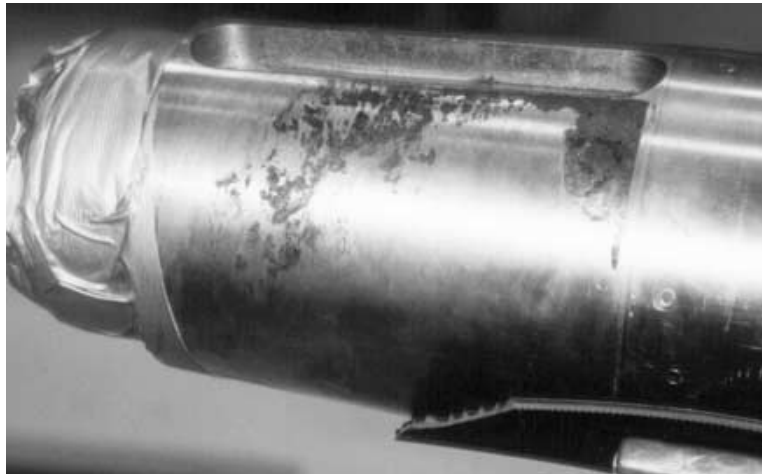
Figure 5-15 Fretting Due to Loose Coupling or Improper Fit Courtesy Jack
