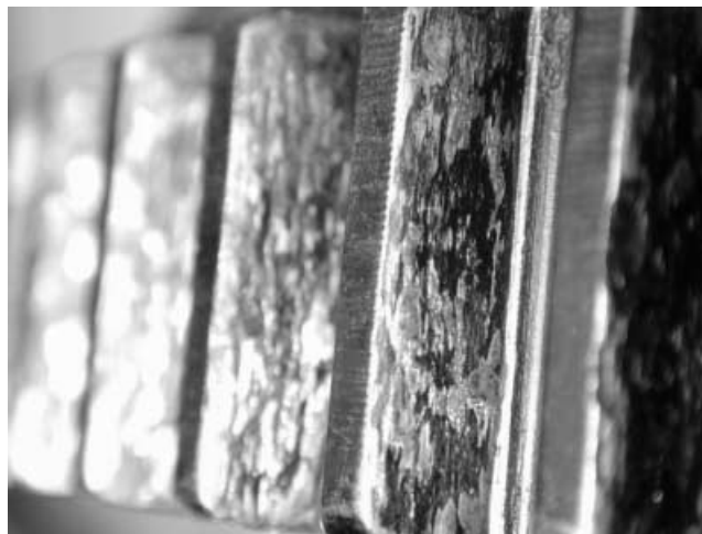
Figure 4-2 Hub Showing Wear on Teeth Courtesy Rota-Tech Inc.
