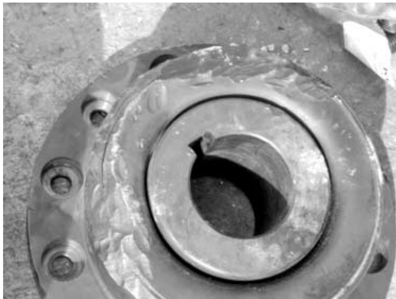
Figure 5-13 Coupling Hub Fit Too Tight for Removal Courtesy Jack
