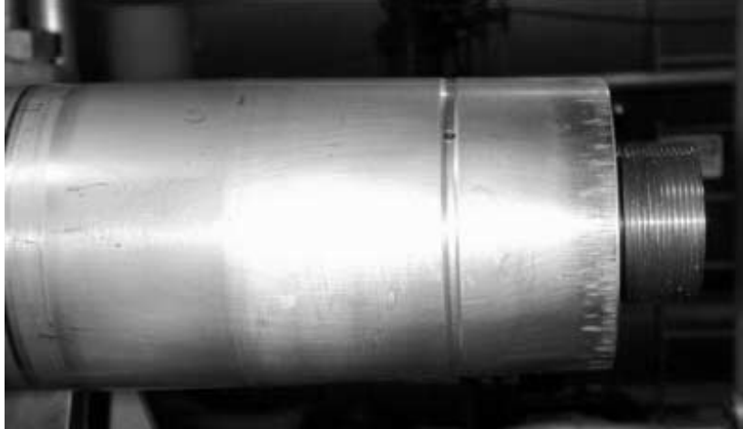
Figure 5-18 Keyless Hydraulically Dilated Coupling Shaft Courtesy Jack
