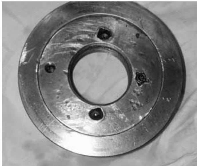
Figure 5-20 Coupling Nut for Hydraulic Coupling Showing Pressure Port, Set Screw, and Spanner Holes Courtesy Jack
