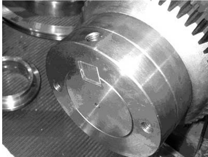
Figure 5-10 Gear Hub with Set Screw Over Key and an Interference Fit Courtesy Jack
