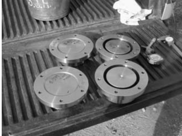
Figure 2-14 Floating Shaft Coupling Components Before Assembly Courtesy Rota-Tech Inc.
