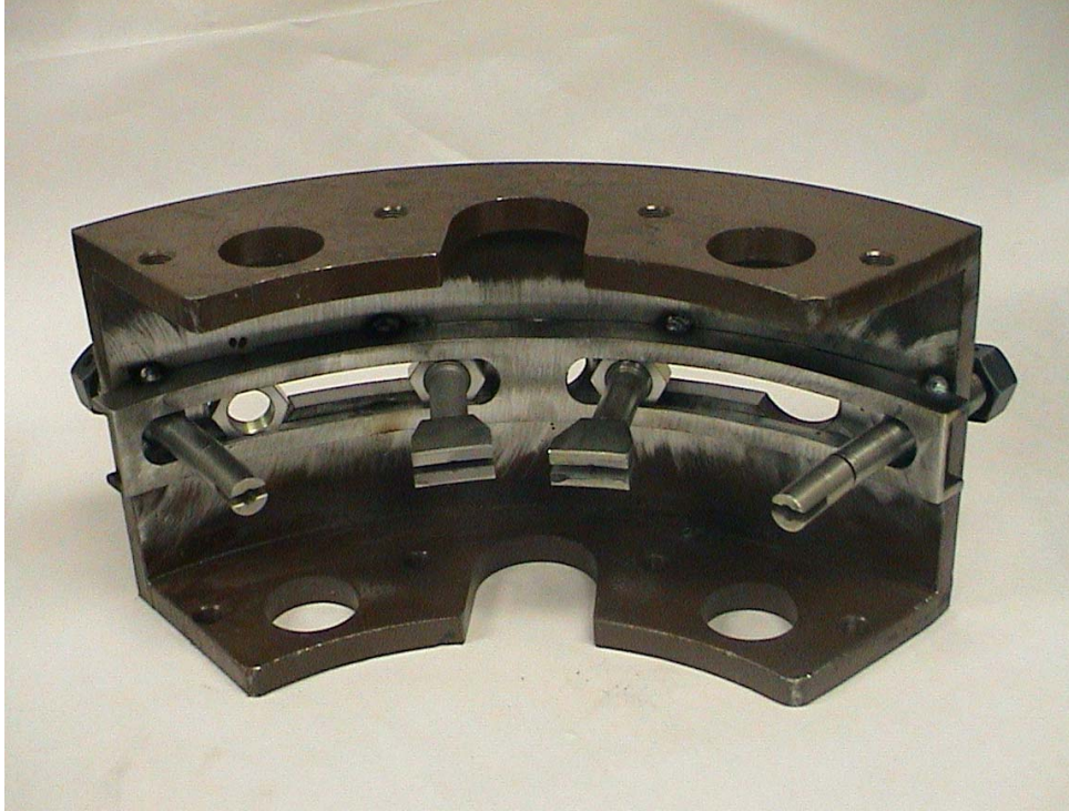
Figure xx – New slotted channel tack welded to fixture.
