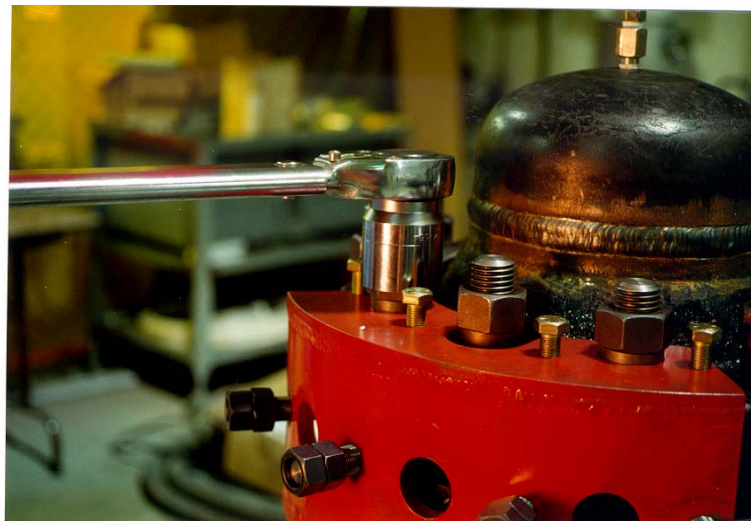
Figure 4-5 Torque Wrench Applying Full Load on Studs But Not on Fixture
