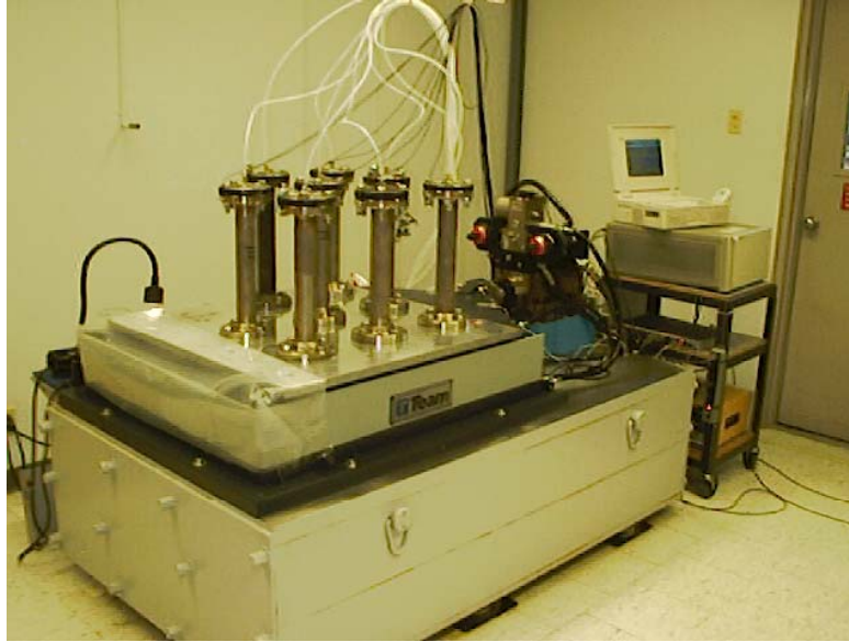
Figure 3-2. Electro-Hydraulic Shaker Table With Eight Specimens On Breadboard (PG&E)
