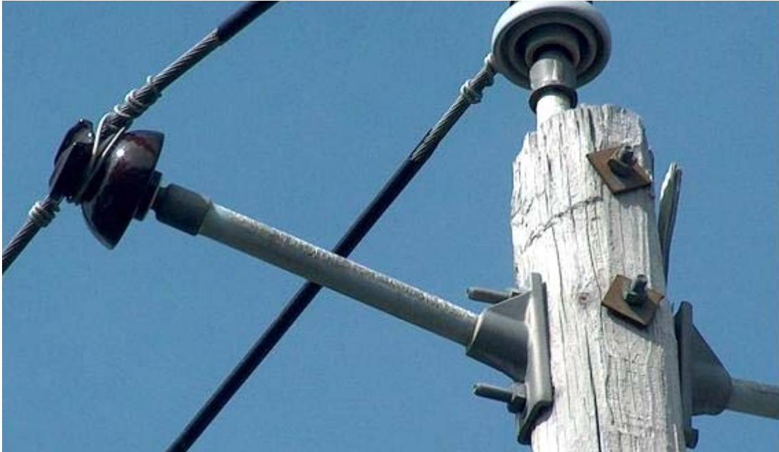
Figure 6-7 Horizontally Mounted Fiberglass Standoff Bracket Showing Surface Degradation
