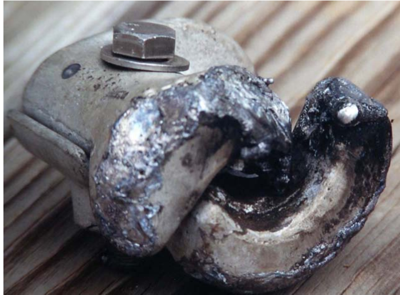
Figure 3-7 An Arc Protective Device That Has “Operated”
