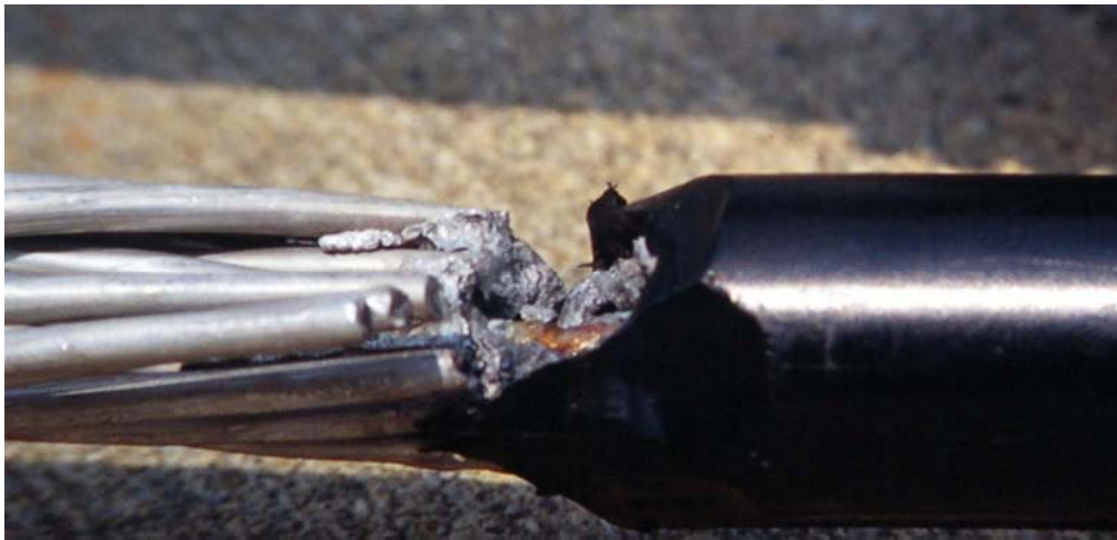
Figure 3-3 Conductor Damage From Arcing Where the Conductor Cover Begins
