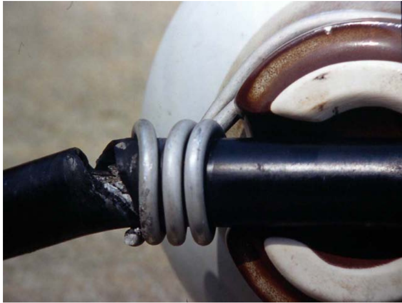
Figure 3-4 Conductor Damage From Arcing
