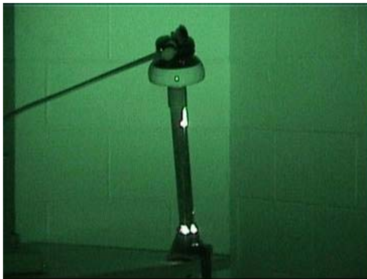
Figure 6-10 Discharges Over the Surface of an Energized Fiberglass Standoff
