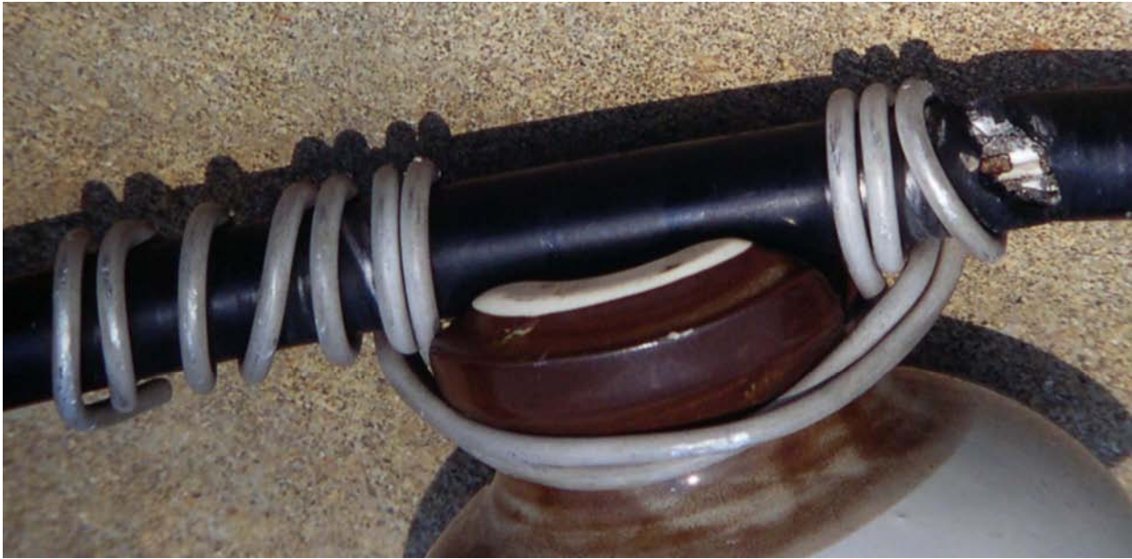
Figure 3-9 Example of Damage on a Covered Conductor From Flashover at the Insulator Tie
