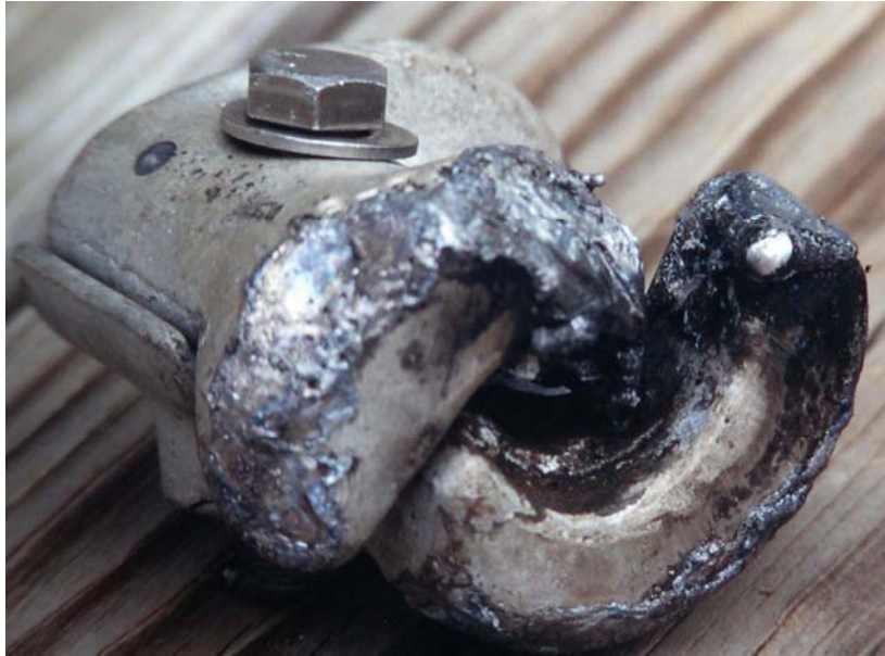
Figure 3-7 An Arc Protective Device That Has “Operated”
