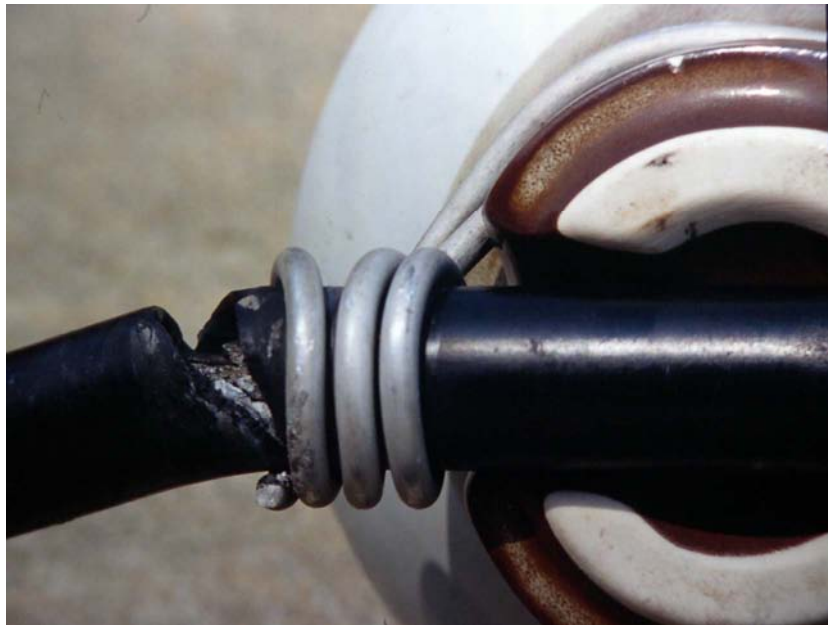
Figure 3-4 Conductor Damage From Arcing
