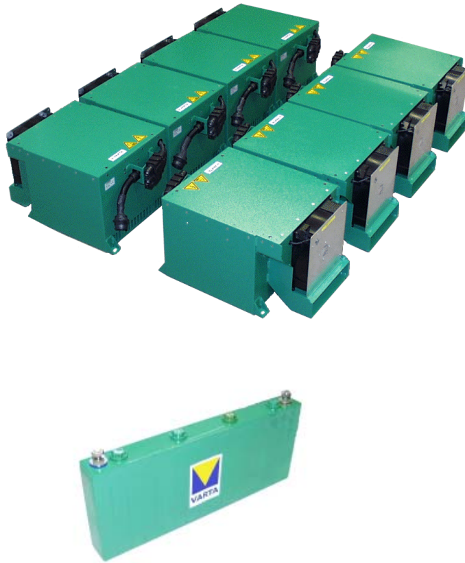
Figure 1-6 VARTA 4-Cell, Plastic-Case, 40 amp-Hour NiMH Module (Below) and Modular Pack System (Above) Based on 32-40 Cell “Blocks”
