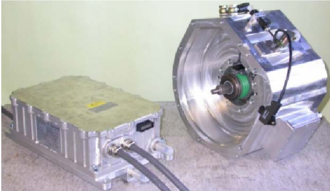
Figure 1-4 ZF Sachs High-Voltage, Permanent Magnet, Synchronous Drive Motor and Motor Control Unit (MCU)
