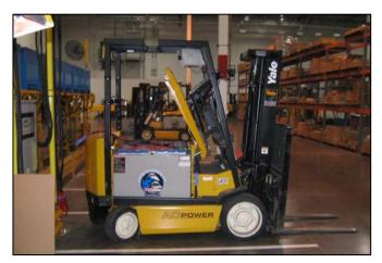
one facility the AC lifts operate from 48V batteries while another facility utilizes lifts that operate from an 80V battery system. The new fast-charger being used by Del Monte Foods is capable of charging both the 48V and 80V fast-charge battery systems associated with this new equipment. With these new 48V and 80V AC forklifts available alongside new DC units, EPRI took advantage of the opportunity for comparison studies of these new technologies.
