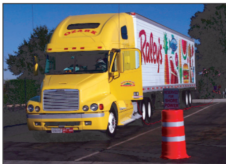
Figure 1. Truck Plugged Into Shorepower at the 49er Truck Stop in Sacramento.
