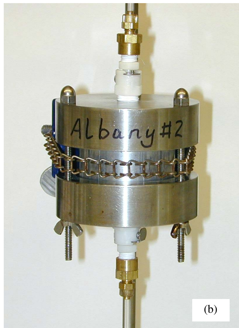
Figure 2-2 a) Glass (Teflon Endplates) and b) Aluminum (Stainless Steel Endplates) Columns used to Measure Coal Tar Residual Saturation
