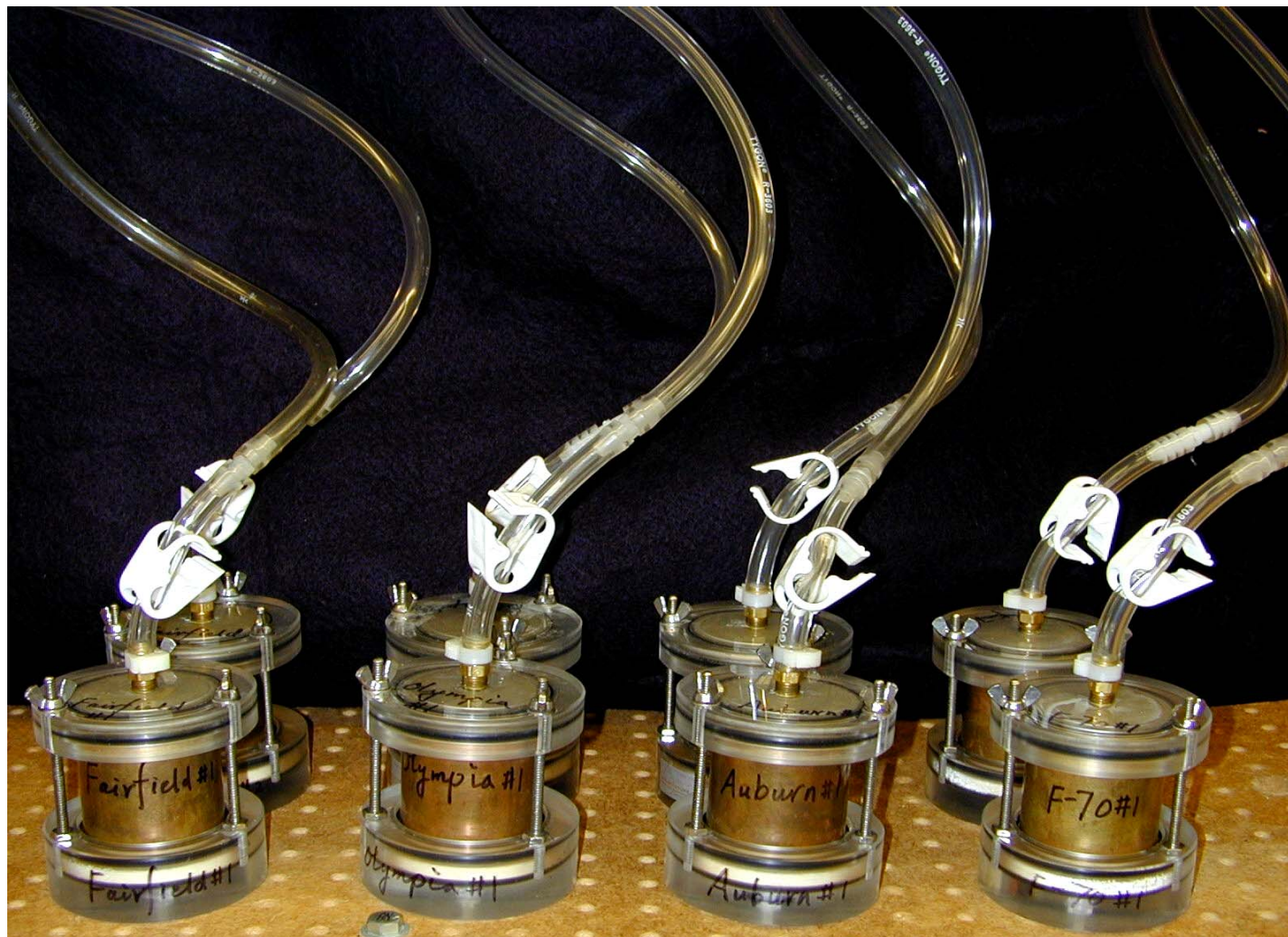
Figure 2-1 Tempe Cells Used to Measure Water Retention Characteristics (Moisture Release Curves) of the Soil Samples
