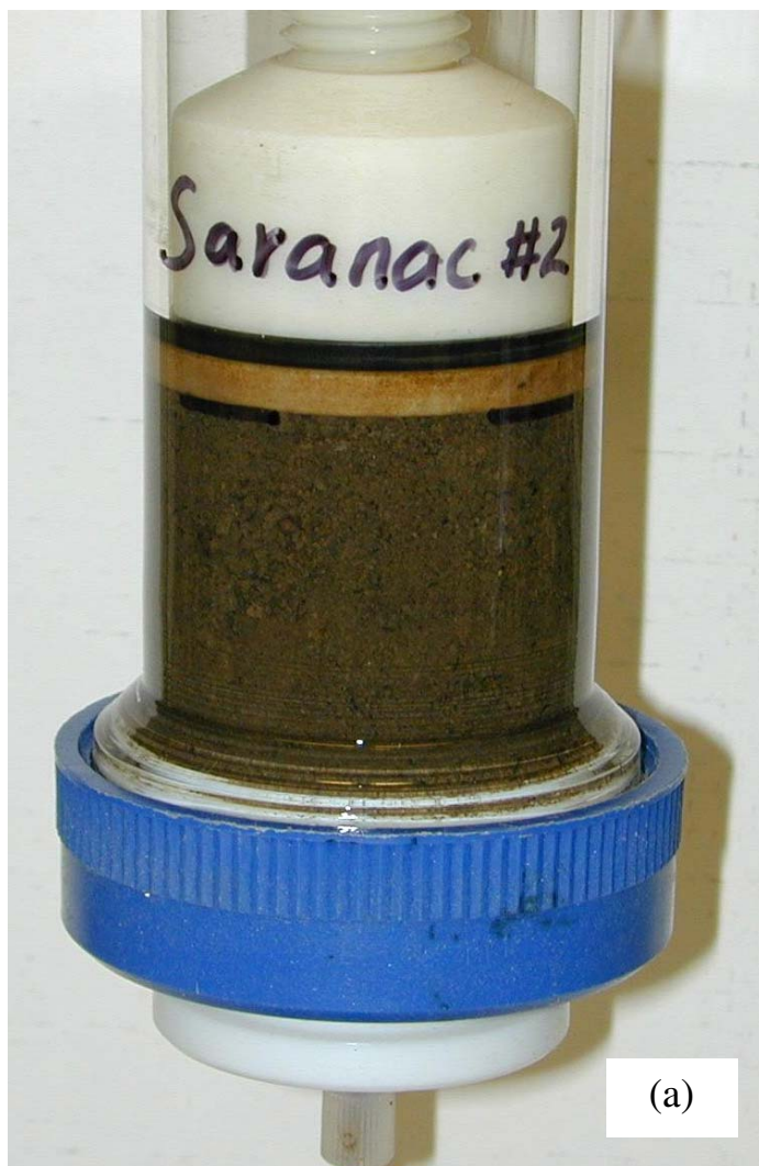
Figure 2-2 a) Glass (Teflon Endplates) and b) Aluminum (Stainless Steel Endplates) Columns used to Measure Coal Tar Residual Saturation
