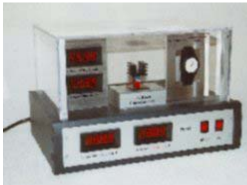
Figure A-2 LPTG Demonstration Device Powering a Wristwatch
