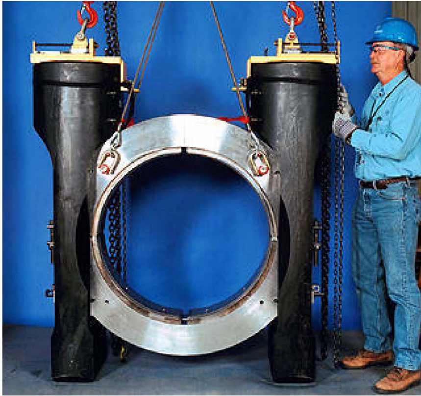
Figure 7-10 VC Summer Hot Leg Nozzle MSIP Tool Details
