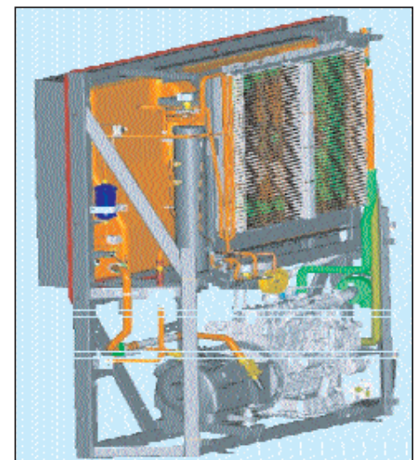
Figure 3. Trailer Mounted Truck Refrigeration Unit.
