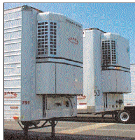
Figure 1. Front View of Refrigerated Highway Trailers With Transport Refrigeration Units (TRUs) Installed.
