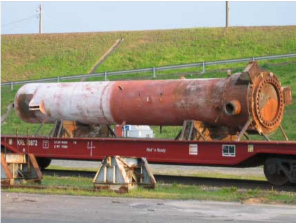
Figure 1 Old Feedwater Heater Ready for Disposal
