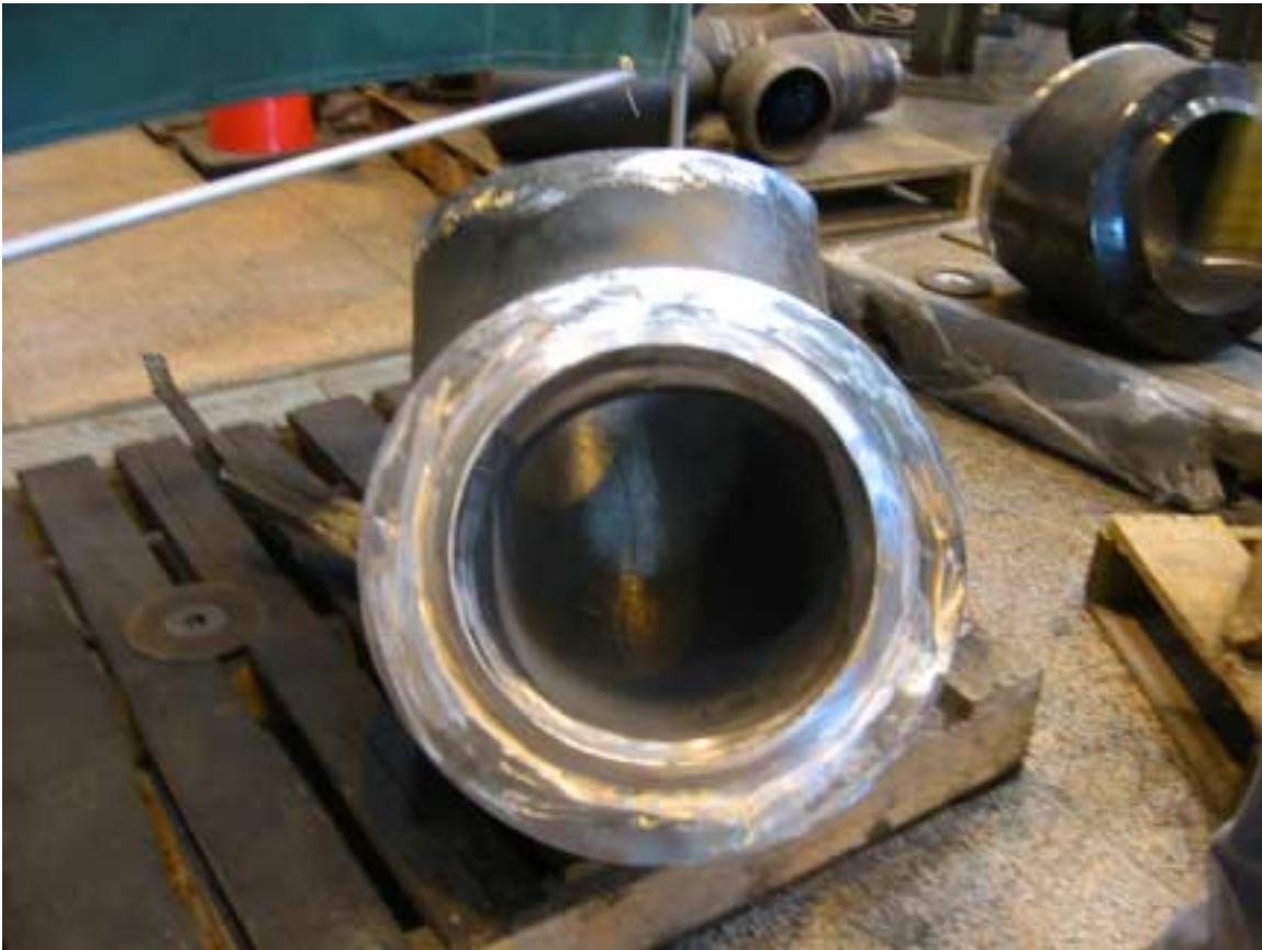
Figure 4 16-Inch Elbow for New Feedwater Line
