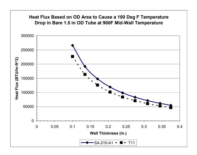
While the temperature distribution is logarithmic, for thin walls it approaches linearity as illustrated in the following figure.
