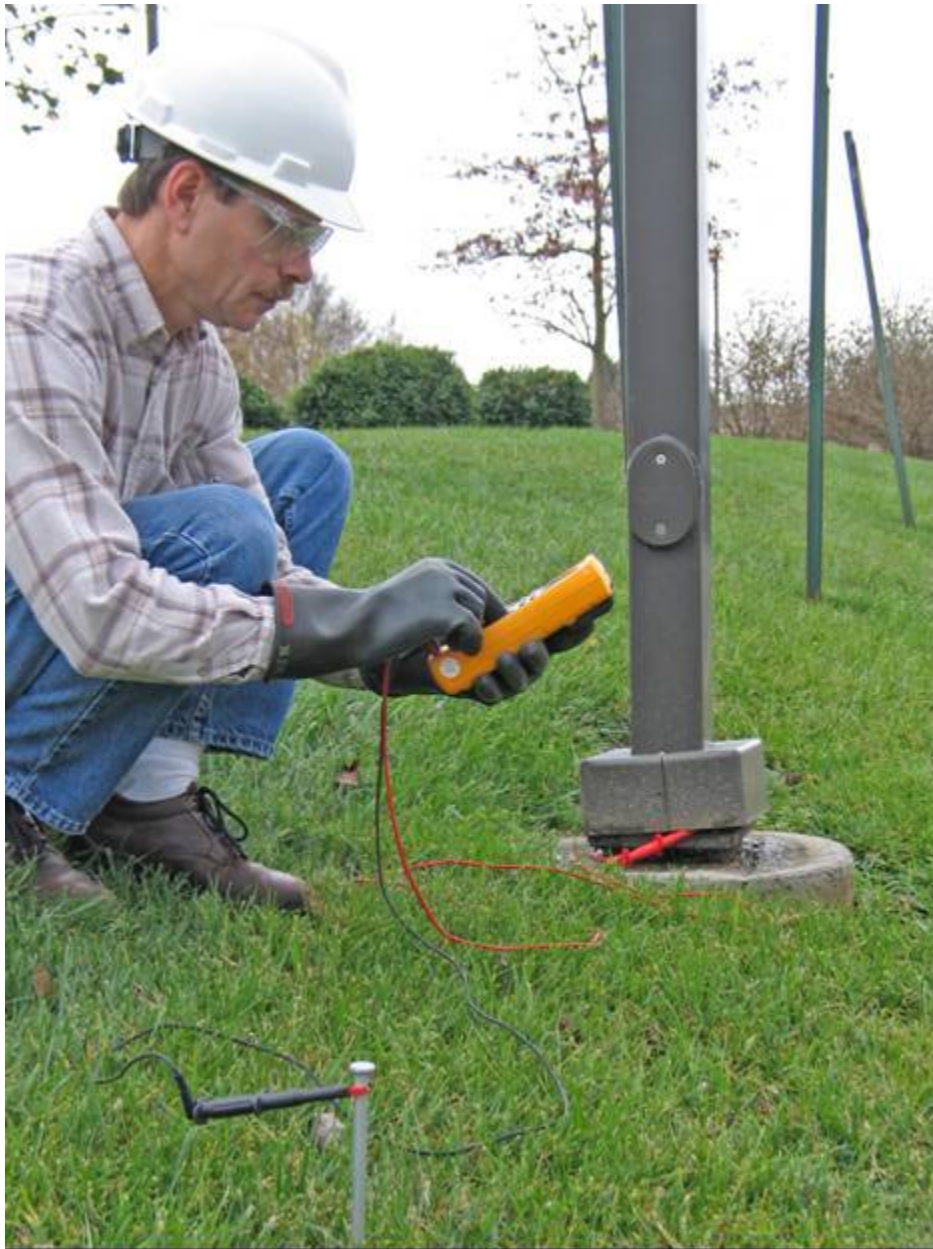
Figure 6-2 Sample Measurements Between a Metal Light Pole and a Reference Ground
