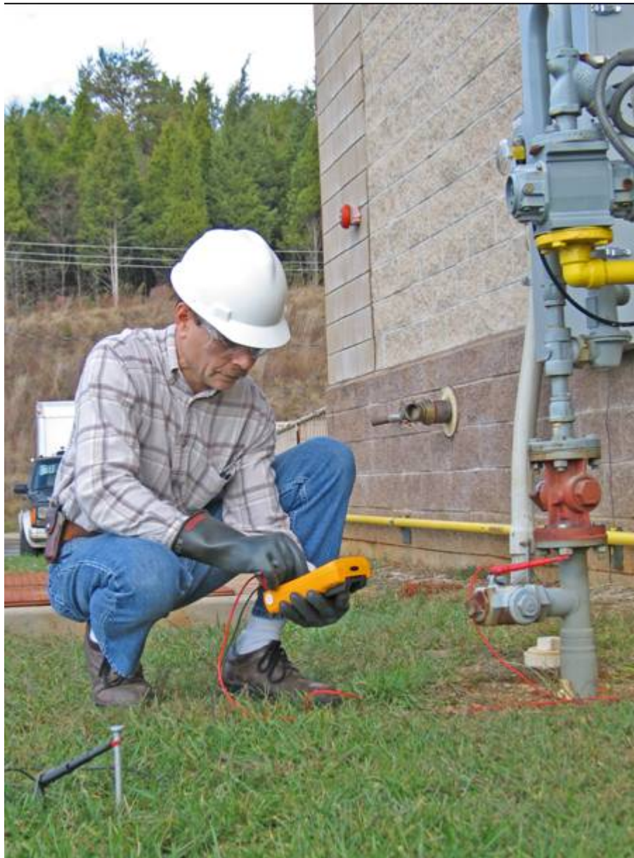
Figure 6-3 Sample Measurements Between a Gas Service Point and a Reference Ground
