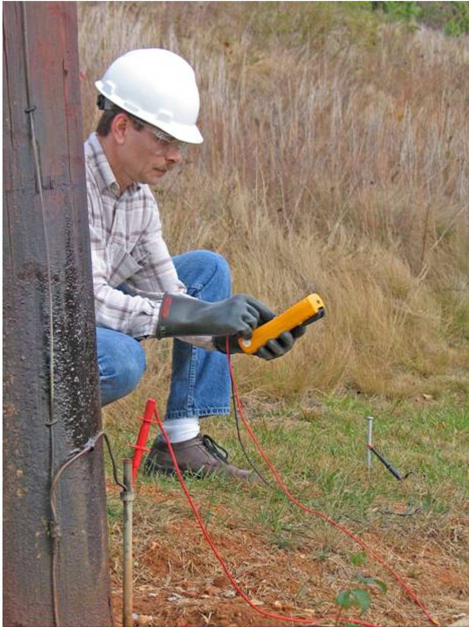
Figure 6-5 Sample Measurements Between a Pole Down Ground and a Reference Ground
