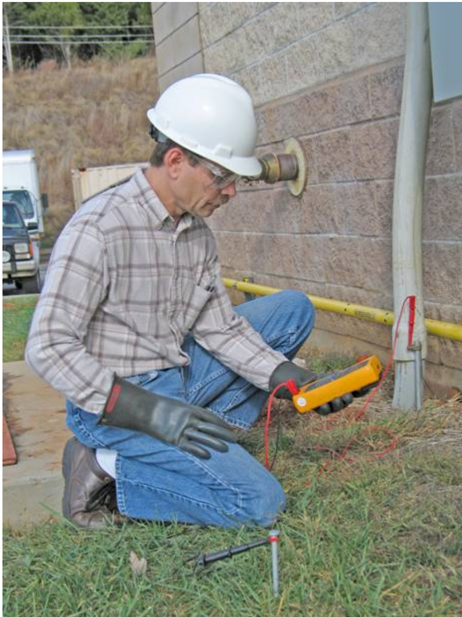
Figure 6-4 Sample Measurements Between a Grounded Meter Base and a Reference Ground
