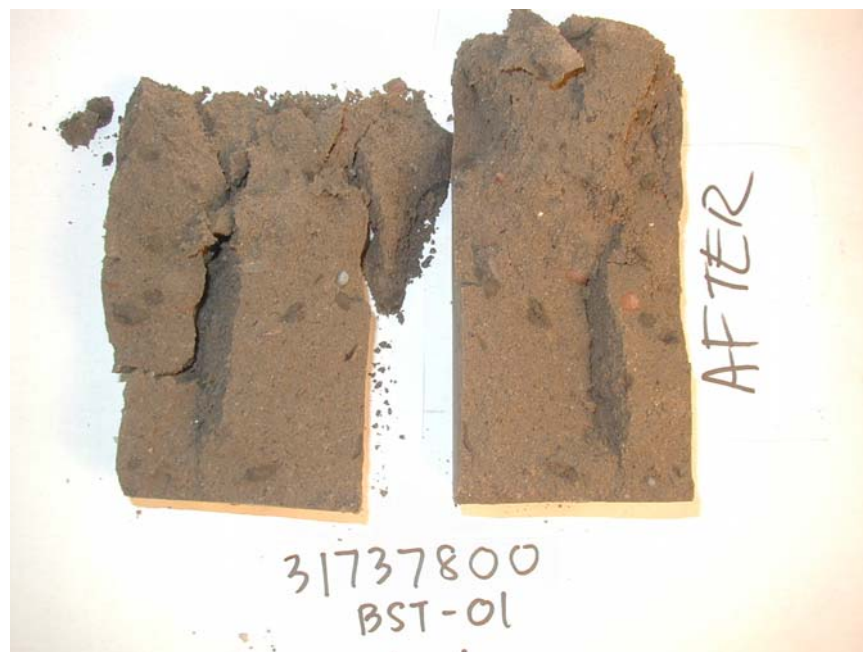
Figure 4-3 Solidified Soil/Cement Cylinder After UCS Test Breakage
