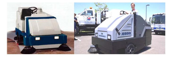
Sweepers, scrubbers and varnishers are used indoors to clean warehouse, manufacturing, and retail store floors, and outdoors to sweep pavement and parking lots.
