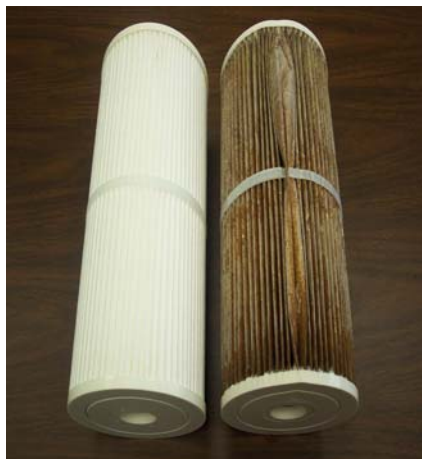
Figure 3-7 Visual Comparison of a Virgin Cartridge (Left) Versus the Test Cartridge after Filtering 2,400 Gallons of Water (Right)
