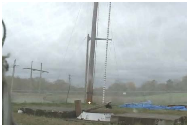
(c) Maximum height reached. Cover remains partially restrained on one side by the passive lip.
