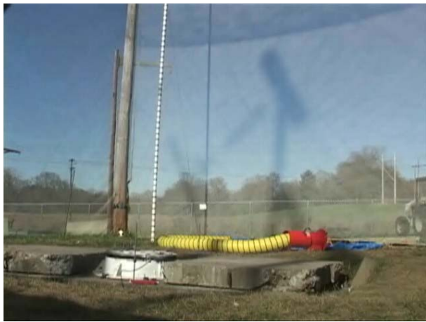
Figure A-3 Event 28. Pin size 0.250". Hydrogen concentration 10%.
