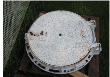
Figure 2-3 Cover #3 – Hinged Saint Gobain solid, white with Stabiloc locking mechanism
