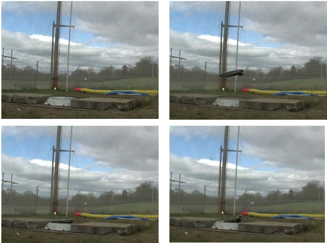
Figure A-1 Event 17. Pin size 0.275". Hydrogen concentration 13%.
