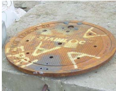
Figure 2-2 Cover #2 – solid, brown, without Stabiloc locking mechanism
