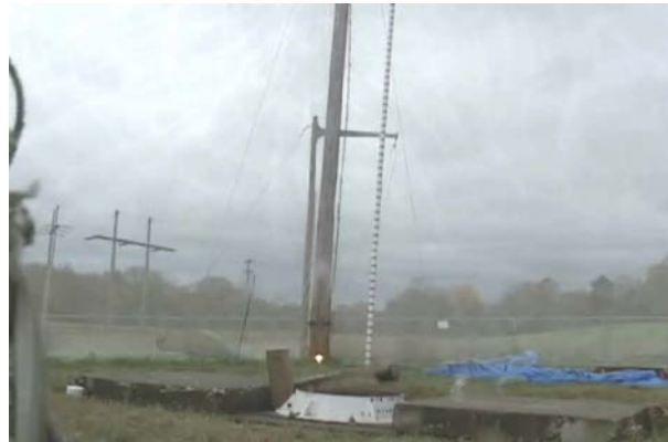
(b) Cover rises unevenly since the restraining mechanism is disengaged on one side.
