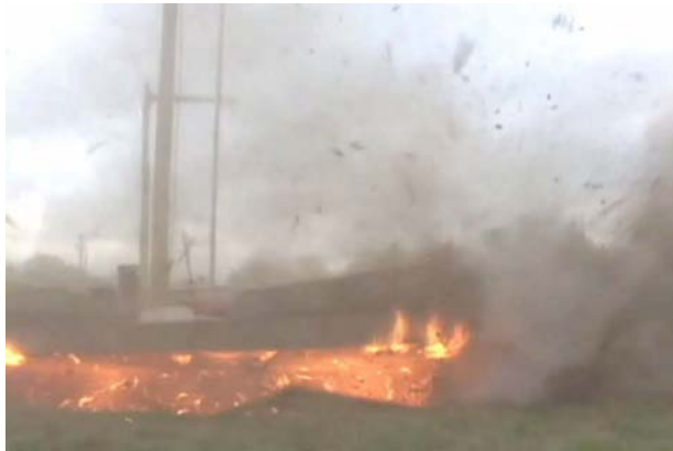
(c) Roof slab rises to about 1.5 ft. Cover remains restrained by the locking mechanism.
