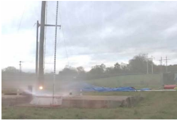
(a) Explosion. Cover rises and partially relieves pressure. Lateral pressure wave is visible.
