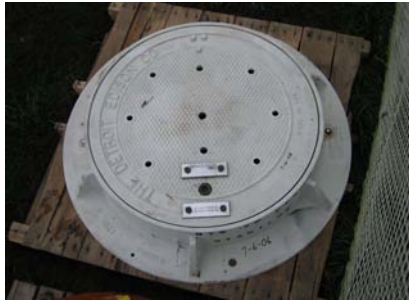
Figure 2-1 Cover #1 – solid, white with Stabiloc locking mechanism
